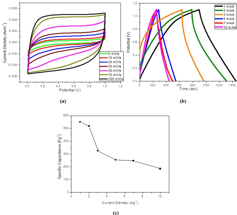
Fig. 14 Electrochemical rate capability performance of the NG-HCD270 electrode. (a) CV curves at different scan rates from 5 to 100  $\text{mV s}^{-1}$ , (b) GCD curves at various current densities of 1–10  $\text{A g}^{-1}$ , and (c) specific capacitance as a function of current density.
