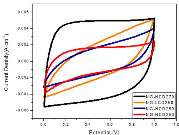
Fig. 11 Cyclic voltammetry curves of graphitic samples.
