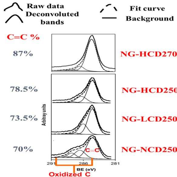
Fig. 3 XPS C1s spectra of graphitic samples.
