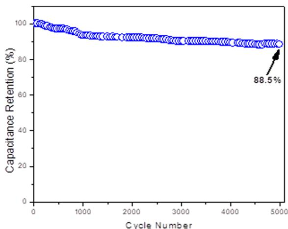
Fig. 15 Cycling stability measurements of the NG-HCD270 supercapacitor electrode.
