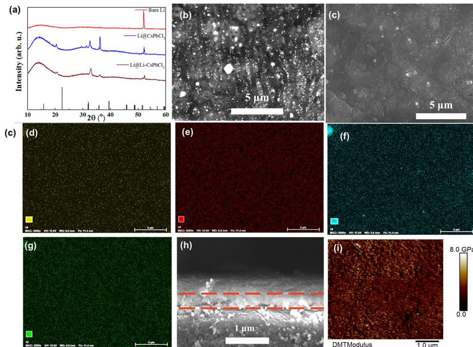
**Fig. 2** (a) XRD patterns of spin-coated  $\text{CsPbCl}_3$  and  $\text{Li-CsPbCl}_3$  on the Li foil surface. (b) and (c) SEM images of the  $\text{Li-CsPbCl}_3$  film coated on Li foil and (d)–(g) corresponding elemental mapping images of Li, Cs, Pb and Cl. (h) Cross-section SEM image of the  $\text{Li-CsPbCl}_3$  film coated on Li foil. (i) AFM Young's modulus mappings of the  $\text{Li-CsPbCl}_3$  film.
