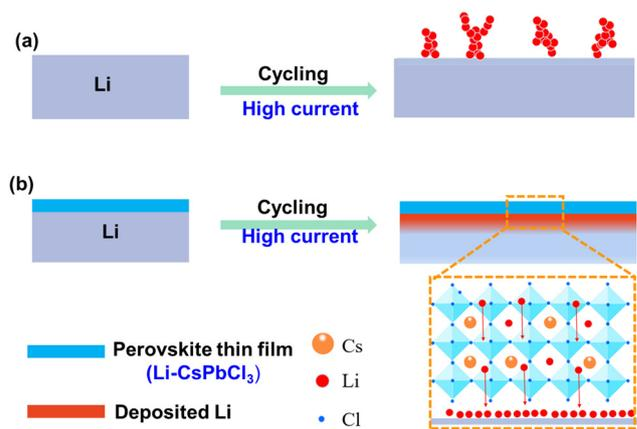
Fig. 1 Schematics of Li plating on (a) bare Li metal and (b) Li metal with artificial  $\text{Li-CSPbCl}_3$  SEI film at high current. The dashed box depicts the mechanism of lithium-ion insertion into the perovskite lattice as well as the formation and deposition process of gradient lithium-ion conductors in the perovskite.
