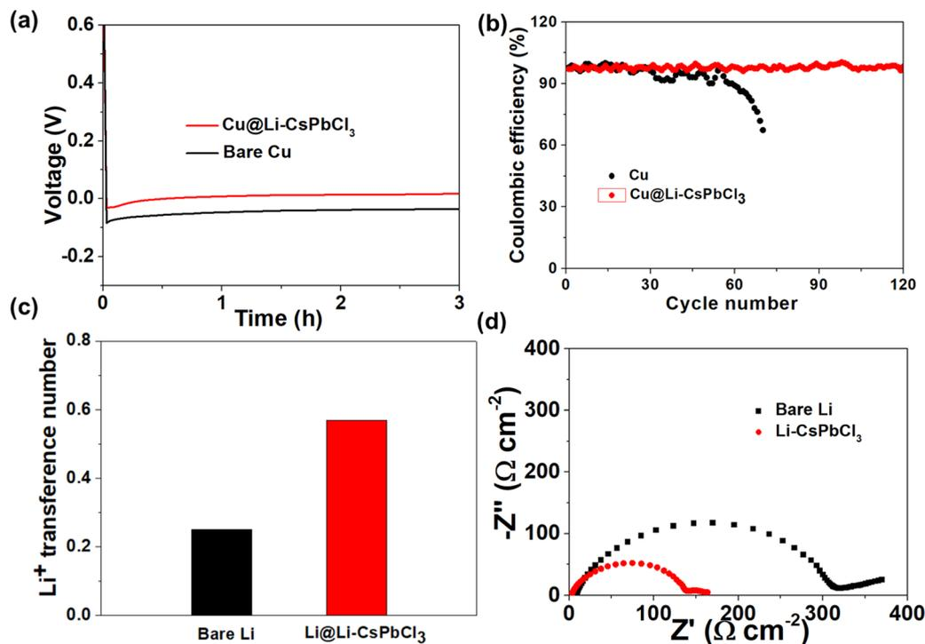
Fig. 3 (a) Voltage profiles of Li plating on Cu@Li-CsPbCl<sub>3</sub> and pristine Cu at 0.2 mA cm<sup>-2</sup>. (b) The cycling performance of Li/Cu and Li/Cu@Li-CsPbCl<sub>3</sub> half cells with a capacity of 1 mA h cm<sup>-2</sup> at 1 mA cm<sup>-2</sup>. (c) The Li<sup>+</sup> transference number for Li and Li@Li-CsPbCl<sub>3</sub> symmetric cells. (d) EIS spectra of Li and Li-CsPbCl<sub>3</sub> symmetrical cells before cycling.
