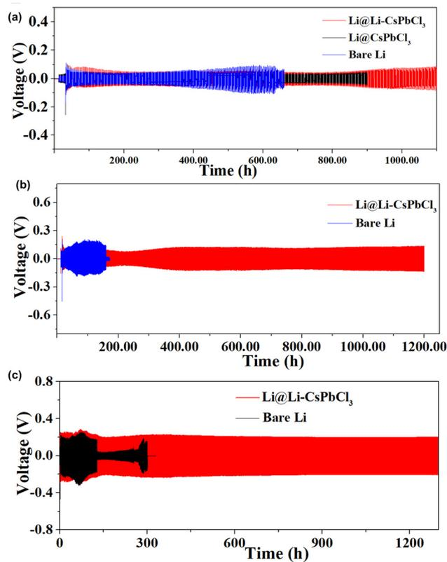
Fig. 4 Voltage-time curves of Li/Li and Li@Li-CsPbCl<sub>3</sub>/Li@Li-CsPbCl<sub>3</sub> symmetric cells with an areal capacity of 1 mA h cm<sup>-2</sup> at a current density of (a) 1 mA cm<sup>-2</sup>, (b) 5 mA cm<sup>-2</sup>, and (c) 10 mA cm<sup>-2</sup>.
