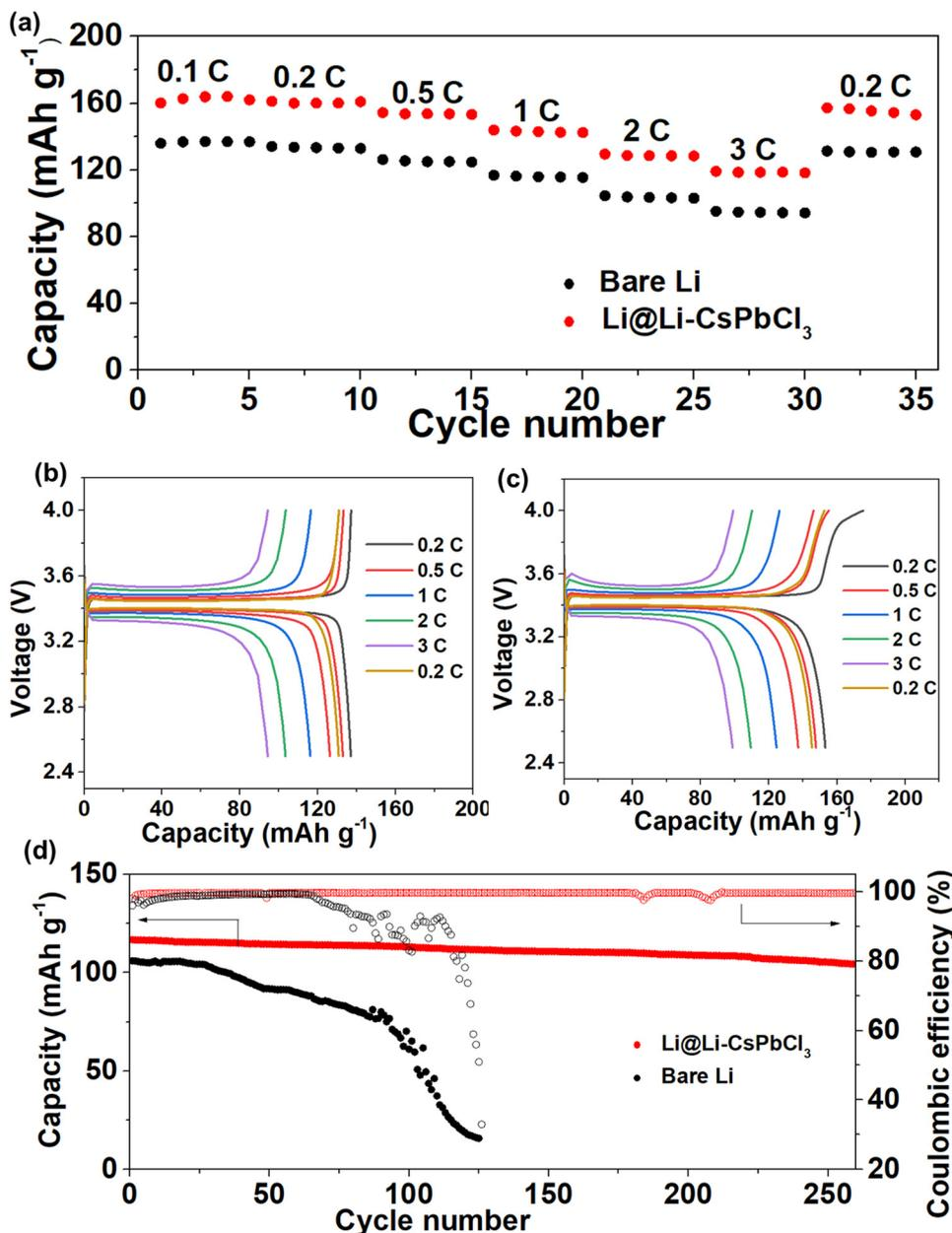
Fig. 6 (a) Rate capability and corresponding charge–discharge profiles of Li/LiFePO<sub>4</sub> cells with (b) bare Li and (c) Li@Li–CsPbCl<sub>3</sub> anodes at different rates from 0.1 to 3C. (d) Long-term cycling stabilities of Li/LiFePO<sub>4</sub> cells with bare Li and Li@Li@Li–CsPbCl<sub>3</sub> anodes at a current density of 3C.
