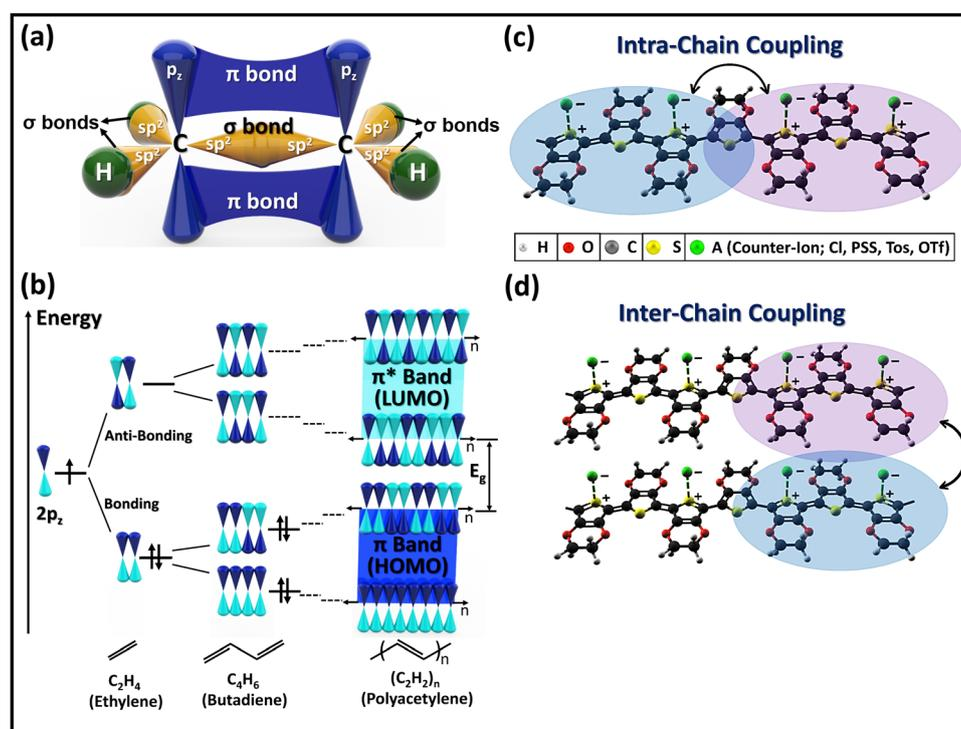
**Fig. 2** Charge transport in conjugated conducting polymers. (a) Schematic illustration of sigma and pi bonds in a conjugated polymer.<sup>8</sup> (b) Change in bandgap as a consequence of bonding and antibonding orbitals in conjugated polymers.<sup>8</sup> (c) Schematic illustration of charge carrier transport through (c) intra-chain coupling,<sup>8</sup> and (d) inter-chain coupling.<sup>8</sup> (a)–(d) Reproduced with permission.<sup>8</sup> Copyright 2020, Elsevier.
