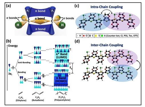
Fig. 2 Charge transport in conjugated conducting polymers. (a) Schematic illustration of sigma and pi bonds in a conjugated polymer.<sup>8</sup> (b) Change in bandgap as a consequence of bonding and antibonding orbitals in conjugated polymers.<sup>8</sup> Schematic illustration of charge carrier transport through (c) intra-chain coupling, and (d) inter-chain coupling. (a)-(d) Reproduced with permission. Copyright 2020, Elsevier.
