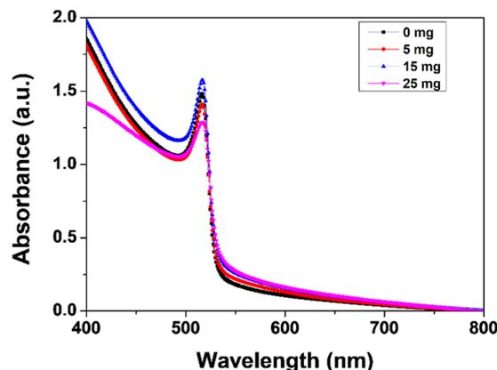
Fig. 5 Absorbance spectra of  $\text{CsPbBr}_3$  with MABr.
