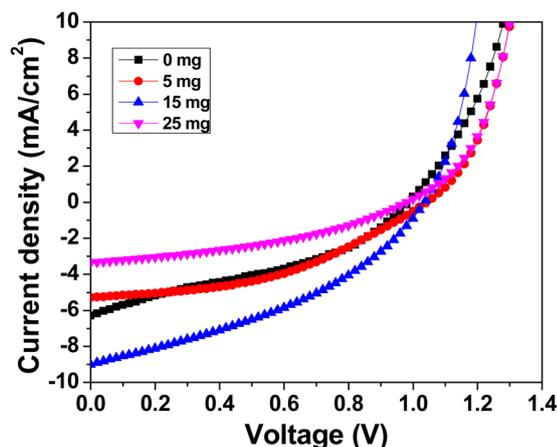
Fig. 8  $J$ - $V$  characteristics of CsPbBr<sub>3</sub> devices with MABr.
