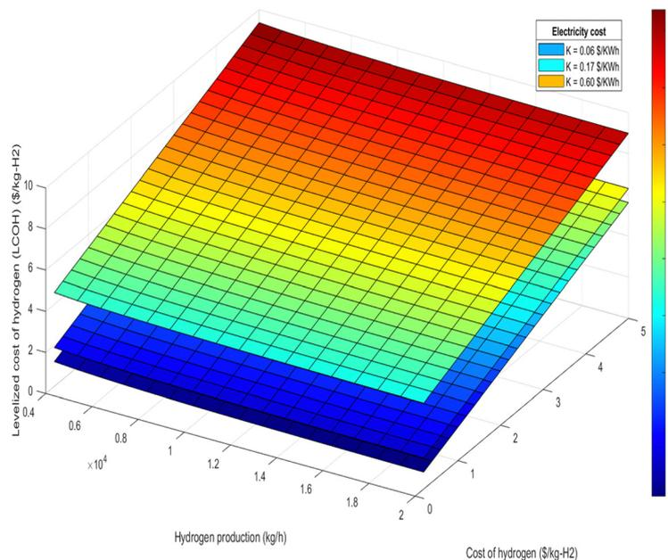
Fig. 12 LCOH at different hydrogen production and different hydrogen cost for 100% renewable electricity mode.
