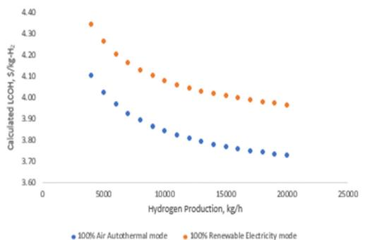
Fig. 17 LCOH at different hydrogen production (ammonia cost used: \$0.550 per kg-NH<sub>3</sub>).
