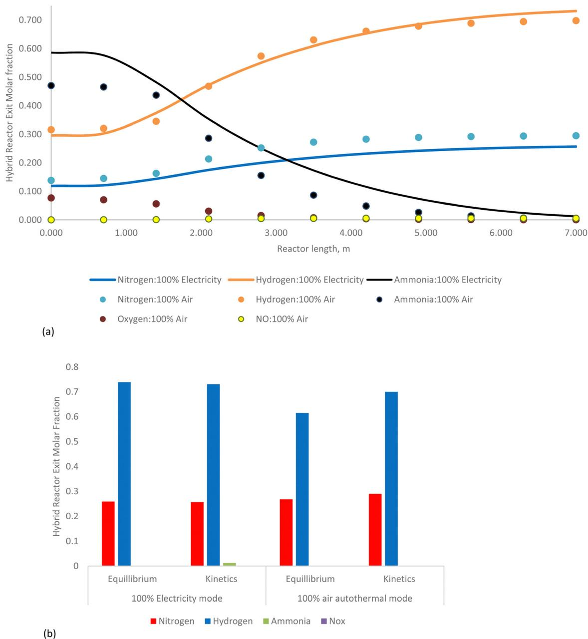
**Fig. 9** (a) Kinetic model for hybrid air-volt ammonia cracker (HAVAC) reactor performance for both 100% renewable electricity and 100% air autothermal mode operation at reactor pressure of 8 barg and temperature of 700 °C. (b) Equilibrium and kinetic model for hybrid air-volt ammonia cracker (HAVAC) reactor for both 100% renewable electricity and 100% air autothermal mode operation at reactor pressure of 8 barg and temperature of 700 °C.
