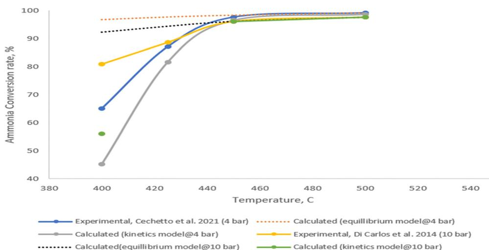
Fig. 2 Conversion vs. temperature for experimental data (Cechetto *et al.* (2021)<sup>62</sup> and Di Carlos *et al.* (2014)<sup>73</sup>), equilibrium model and kinetic model across temperatures ranging from 400 °C to 500 °C and pressures of 4 barg and 10 barg.
