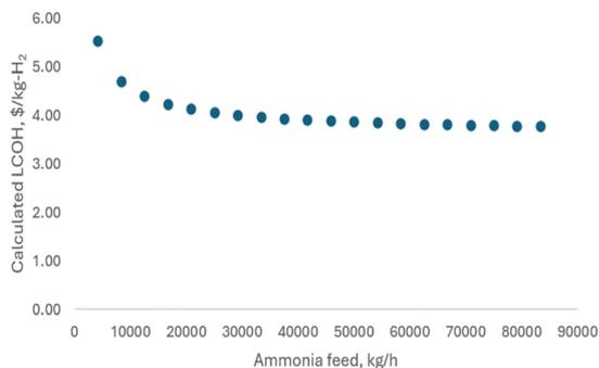
Fig. 18 LCOH at different ammonia feed (ammonia cost used: \$0.550 per kg-NH<sub>3</sub>).
