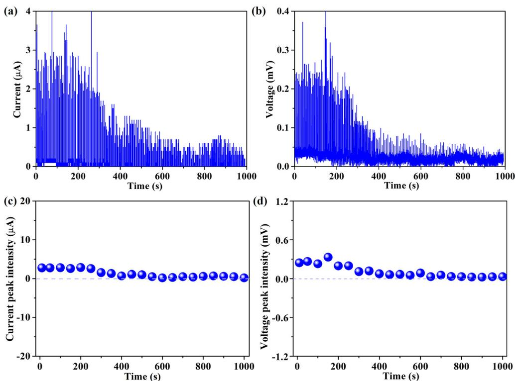
Fig. 8 Stability of (a) current and (b) voltage by persistently dropping 0.6 M NaCl aqueous solution on the 94 wt% G-CB/PVC film at an injection velocity of 60 mL h<sup>-1</sup>. The durability of (c) current and (d) voltage outputs.
