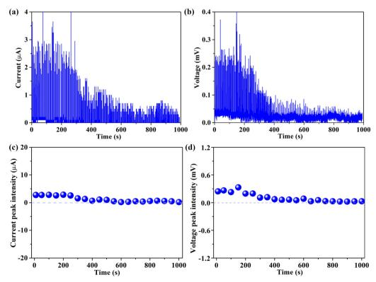
Fig. 8 Stability of (a) current and (b) voltage by persistently dropping 0.6 M NaCl aqueous solution on the 94 wt% G-CB/PVC film at an injection velocity of  $60 \text{ mL h}^{-1}$ . The durability of (c) current and (d) voltage outputs.
