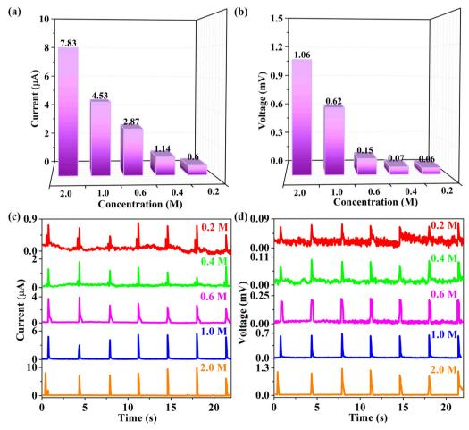
Fig. 6 Histogram of (a) current and (b) voltage values by dropping NaCl aqueous solution with different concentrations on the 94 wt% G-CB/PVC film at an injection velocity of 60 mL  $h^{-1}$ . (c) Current and (d) voltage signals.
