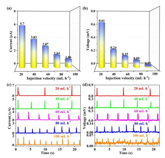
Fig. 4 Histograms of (a) current and (b) voltage values by dropping 0.6 M NaCl aqueous solution on the 94 wt% G-CB/PVC composite film at different intervals of two droplets by controlling the injection velocities. (c) Current and (d) voltage signals.
