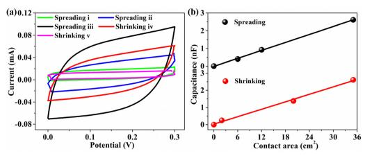
Fig. 5 (a) CV curves for the symmetric dummy cells with 94 wt% G-CB/PVC film 0.6 M NaCl 94 wt% G-CB/PVC film architecture. (b) Linear plots of the capacitance as a function of the contact area between a raindrop and the 94 wt% G-CB/PVC composite film.
