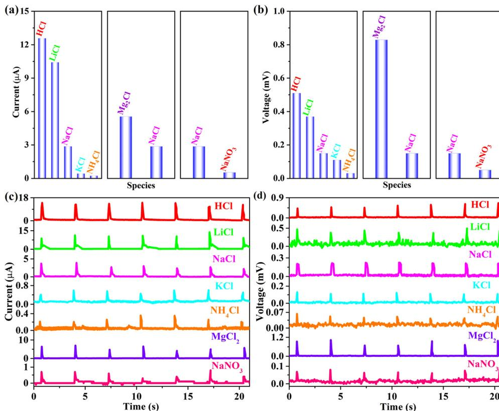
Fig. 7 Histograms of (a) current and (b) voltage values by dropping 0.6 M chlorides and  $\text{NaNO}_3$  aqueous solution on the 94 wt% G-CB/PVC film at an injection velocity of  $60 \text{ mL h}^{-1}$ . (c) Current and (d) voltage signals.
