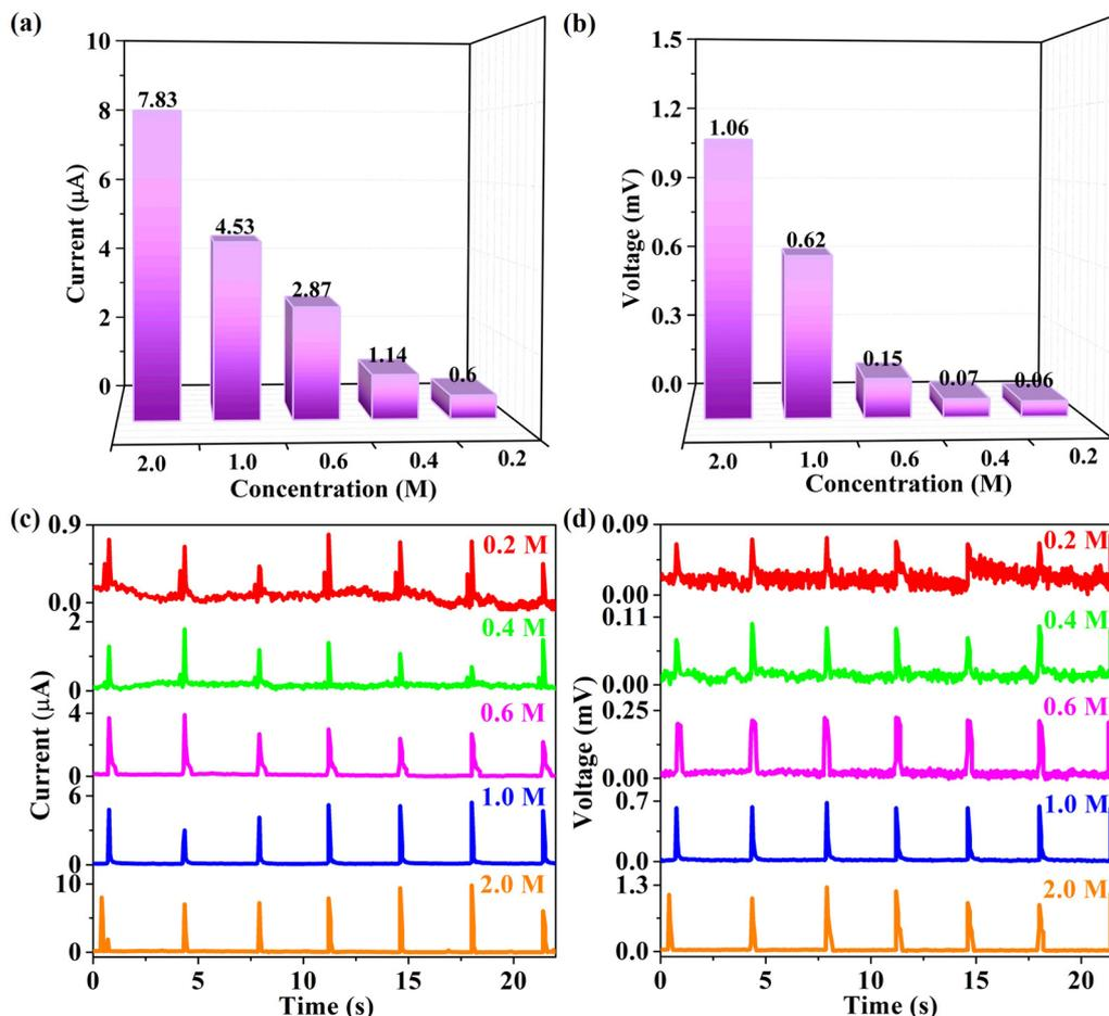
Fig. 6 Histogram of (a) current and (b) voltage values by dropping NaCl aqueous solution with different concentrations on the 94 wt% G-CB/PVC film at an injection velocity of 60 mL h<sup>-1</sup>. (c) Current and (d) voltage signals.
