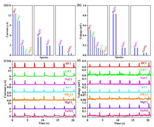
Fig. 7 Histograms of (a) current and (b) voltage values by dropping 0.6 M chlorides and NaNO3 aqueous solution on the 94 wt% G-CB/PVC film at an injection velocity of 60 mL h<sup>-1</sup>. (c) Current and (d) voltage signals.
