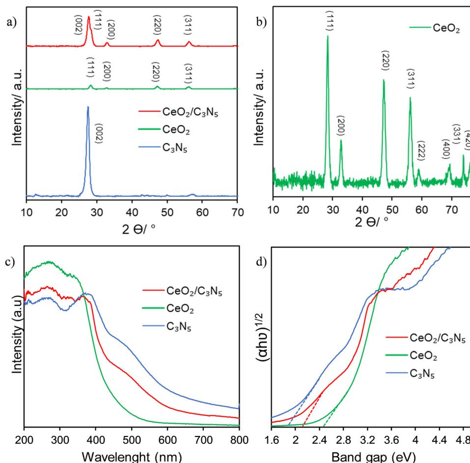
Fig. 1 (a) XRD patterns of C<sub>3</sub>N<sub>5</sub>, CeO<sub>2</sub> and CeO<sub>2</sub>/C<sub>3</sub>N<sub>5</sub> composites. (b) XRD patterns of CeO<sub>2</sub>. (c) UV-vis absorbance spectra and (d) optical band gap using relative Tauc plots.
