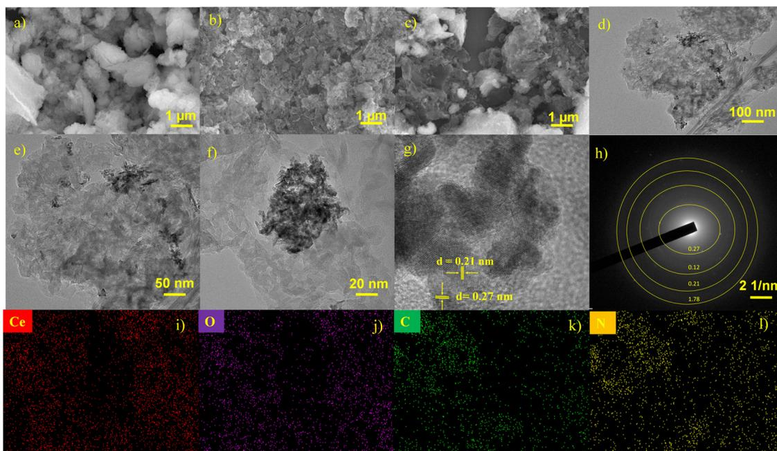
Fig. 2 SEM images of (a)  $\text{CeO}_2$ , (b)  $\text{C}_3\text{N}_5$ , and (c)  $\text{CeO}_2/\text{C}_3\text{N}_5$  composites; (d)–(g) high-resolution TEM (HRTEM) images of  $\text{CeO}_2/\text{C}_3\text{N}_5$  composites; (h) clear fringes with lattice spacings. (i)–(l) EDS mapping images of Ce, O, C, and N elements.
