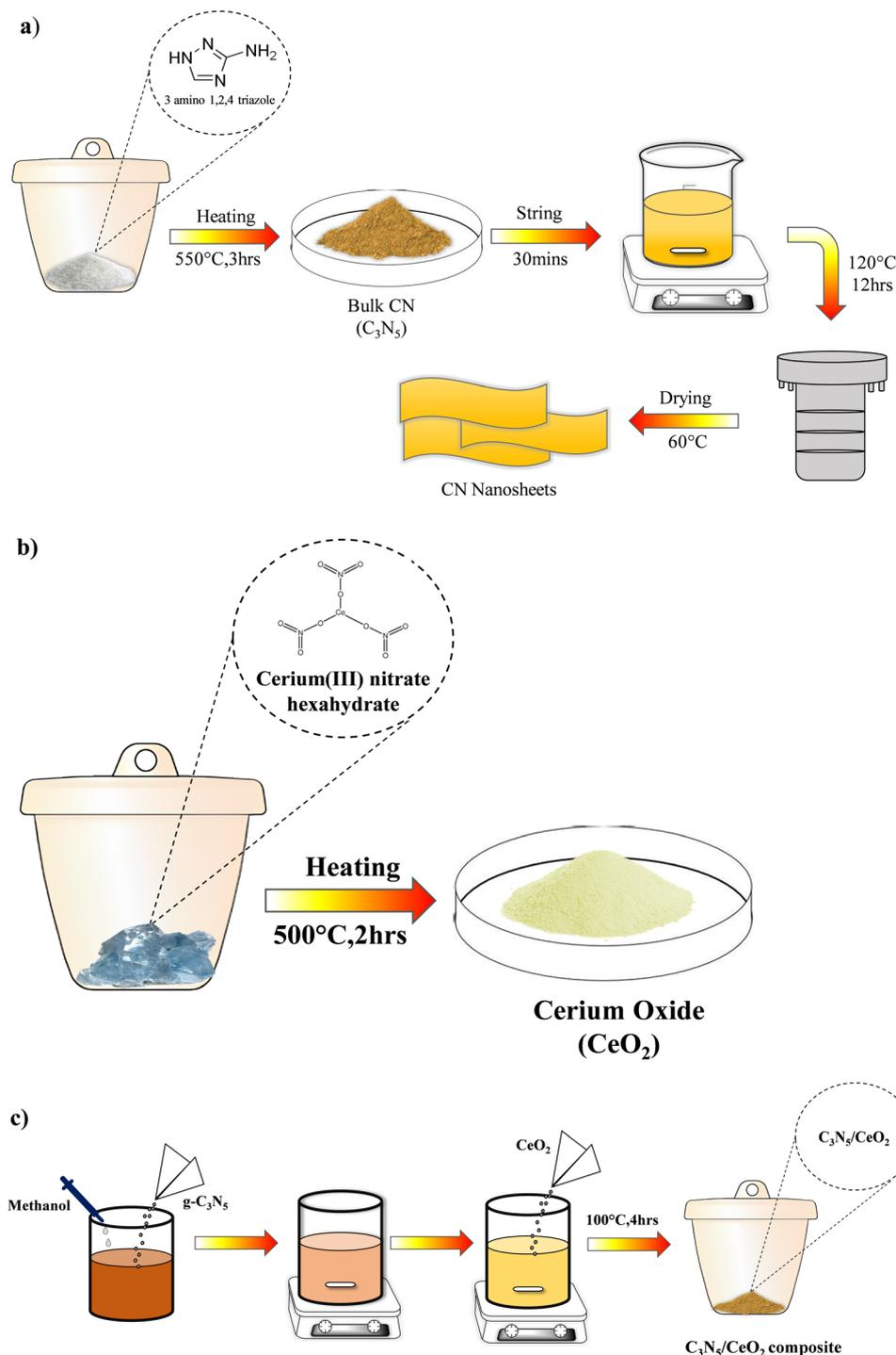
**Scheme 1** (a). Schematic representation of the synthesis of C<sub>3</sub>N<sub>5</sub>. (b) Schematic representation of the synthesis of CeO<sub>2</sub>. (c) Schematic representation of the synthesis of the C<sub>3</sub>N<sub>5</sub>/CeO<sub>2</sub> composite.
