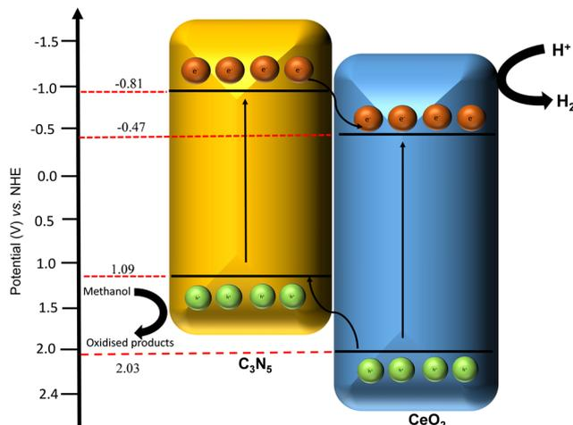
Fig. 6 Plausible mechanism of the  $\text{CeO}_2/\text{C}_3\text{N}_5$  catalyst.
