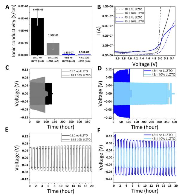
Fig. 4 (A) Ionic conductivities and (B) LSV scans (Cu/electrolyte/Li cells from OCV to 6 V) of four electrolytes at room temperature. Galvanostatic cycling of Li/electrolyte/Li symmetric cells at 0.2 mA cm<sup>-2</sup> at 50 °C with high Li salt concentration (18:1) (C) and (E), and low Li salt concentration (43:1) (D) and (F) solid-state electrolytes
