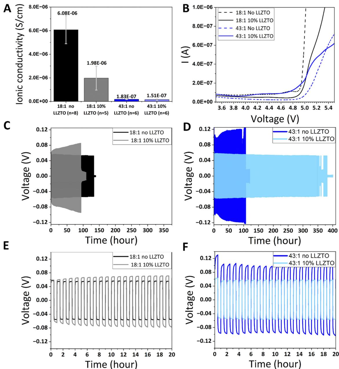
Fig. 4 (A) Ionic conductivities and (B) LSV scans (Cu/electrolyte/Li cells from OCV to 6 V) of four electrolytes at room temperature. Galvanostatic cycling of Li/electrolyte/Li symmetric cells at  $0.2 \text{ mA cm}^{-2}$  at  $50^\circ\text{C}$  with high Li salt concentration (18 : 1) (C) and (E), and low Li salt concentration (43 : 1) (D) and (F) solid-state electrolytes.
