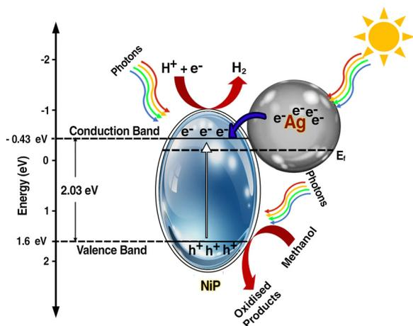
Fig. 8 Plausible photocatalytic water splitting mechanism of Ag-CL/Ni-P.
