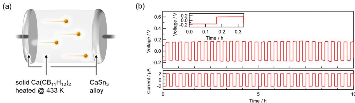
Fig. 3 (a) Illustration of symmetric cell setup (CaSn<sub>3</sub> alloy|CMC heated at 433 K). (b) Voltage response (top), applied current, and voltage response for 0–20 min (inset) in galvanostatic test using CaSn<sub>3</sub> symmetric cell.
