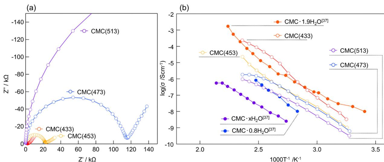
Fig. 2 (a) Nyquist plots at 423 K of CMC heat-treated at different temperatures ( $T = 433, 453, 473,$  and  $513$  K). (b) Arrhenius plots of CMC (433–513) and hydrated CMCs.<sup>37</sup>
