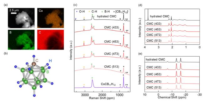
Fig. 1 (a) SEM image and EDS analysis of CMC particles. (b) Molecular model of  $[CB_{11}H_{12}]^-$  anion. (c) Raman spectra of  $CsCB_{11}H_{12}$ , hydrated CMC, and CMC heat-treated at different temperatures (T = 433, 453, 473, and 513 K). (d) <sup>1</sup>H and (e) <sup>11</sup>B NMR spectra of hydrated CMC and CMC (433–513 K).
