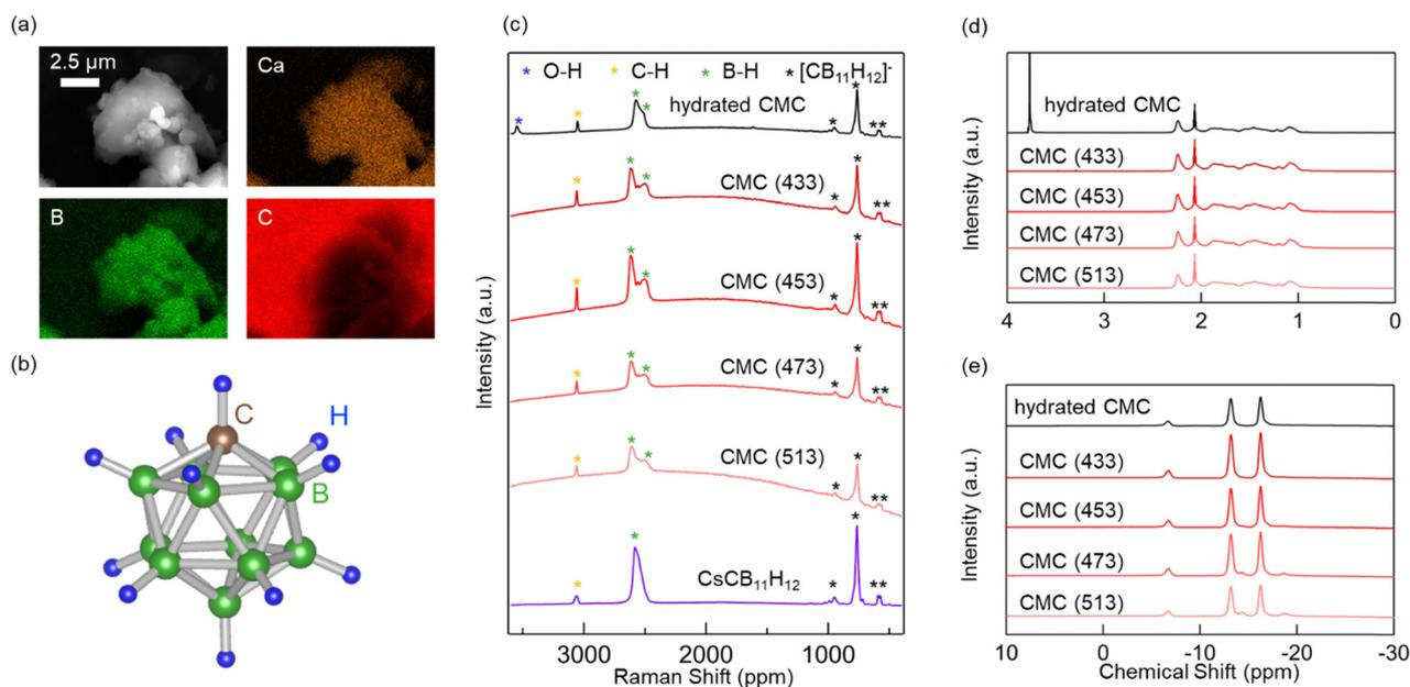
**Fig. 1** (a) SEM image and EDS analysis of CMC particles. (b) Molecular model of  $[\text{CB}_{11}\text{H}_{12}]^-$  anion. (c) Raman spectra of  $\text{CsCB}_{11}\text{H}_{12}$ , hydrated CMC, and CMC heat-treated at different temperatures ( $T = 433$ ,  $453$ ,  $473$ , and  $513\ \text{K}$ ). (d)  $^1\text{H}$  and (e)  $^{11}\text{B}$  NMR spectra of hydrated CMC and CMC ( $433$ – $513\ \text{K}$ ).
