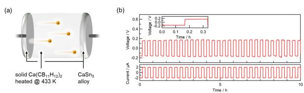
Fig. 3 (a) Illustration of symmetric cell setup (CaSn<sub>3</sub> alloy|CMC heated at 433 K). (b) Voltage response (top), applied current, and voltage response for 0-20 min (inset) in galvanostatic test using CaSn<sub>3</sub> symmetric cell.
