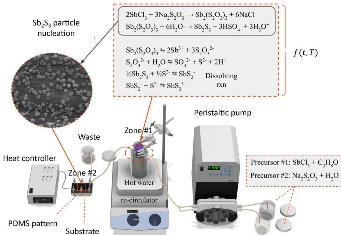
Fig. 2 Process schematics for  $\text{Sb}_2\text{S}_3$  thin films.
