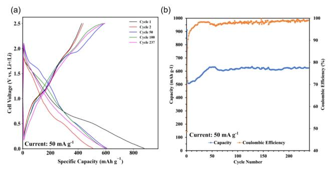
Fig. 15 GCD results. (a) Specific capacity vs. cell voltage; (b) coulombic efficiency and discharge capacity vs. cycle number.
