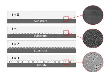
Fig. 7 Heterogeneous nucleation Sb<sub>2</sub>S<sub>3</sub> film.
