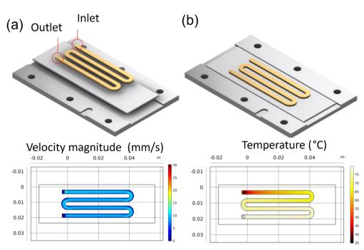
Fig. 3 COMSOL simulation results for reaction inlet velocity of 14.9 mm s<sup>-1</sup> at 35 °C on an 80 °C heating plate: (a) the velocity profile at center line, (b) the surface temperature.
