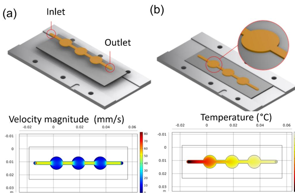
Fig. 4 COMSOL simulation results for reaction inlet velocity of  $14.9 \text{ mm s}^{-1}$  at  $20 \text{ }^\circ\text{C}$  on an  $80 \text{ }^\circ\text{C}$  heating plate: (a) the velocity profile at center line, (b) the surface temperature.
