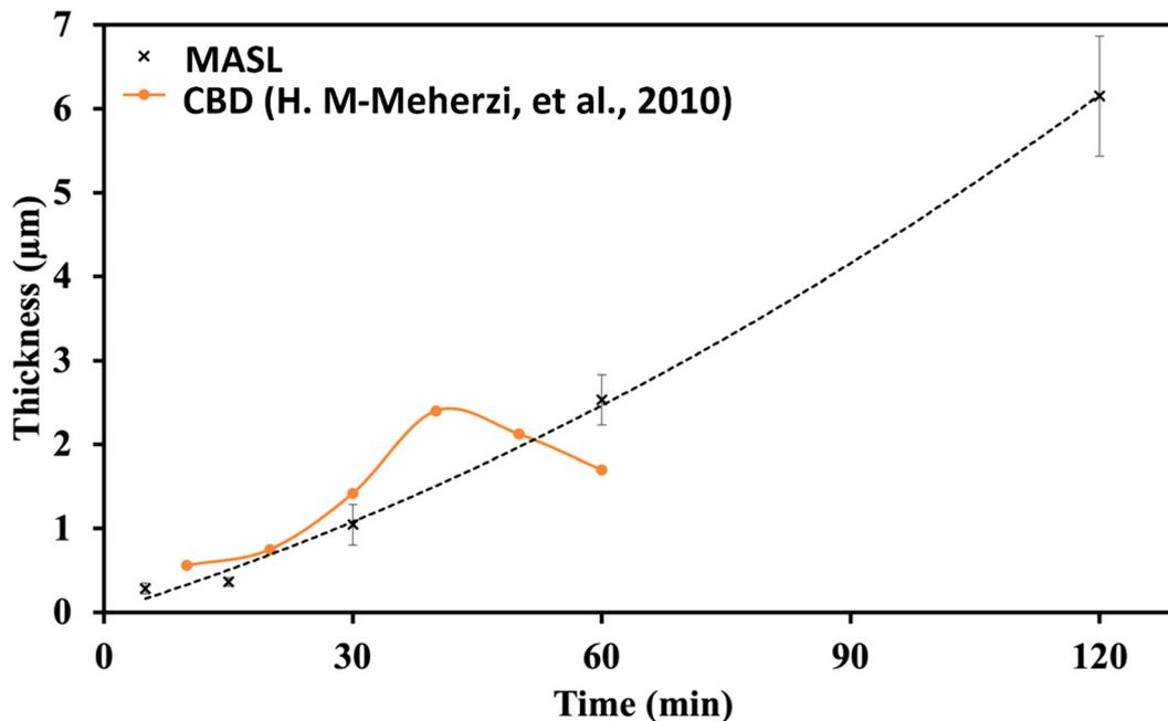
Fig. 9 Thickness vs. time comparison of MASL (this study) and chemical bath deposition.<sup>39</sup>
