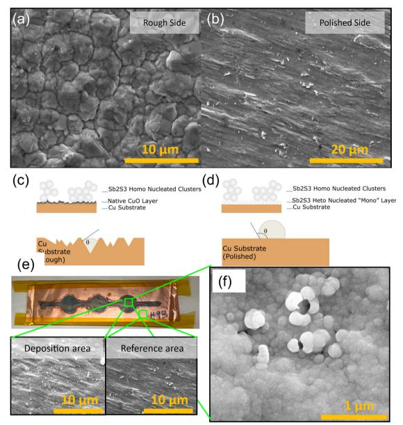
Fig. 13 SEM images of uncoated MTI Cu foil and nucleation barrier theory diagrams. (a) Rough side, (b) polished side, (c) native oxide barrier to heterogenous nucleation, (d) removed native oxide nucleation, (e) optical image of the deposited film on polished and cleaned Cu foil and SEM images of deposited and non-deposited areas, (f) Sb<sub>2</sub>S<sub>3</sub> film deposited on polished copper foil substrates followed by HCl cleaning.
