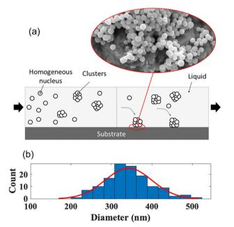
Fig. 6 (a) Homogeneous nucleation  $\mathrm{Sb}_2\mathrm{S}_3$  nanoparticles and (b) size distribution.
