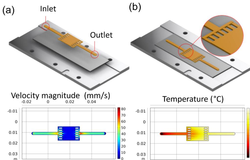
Fig. 5 COMSOL simulation results for reaction inlet velocity of  $44 \text{ mm s}^{-1}$  at  $40 \text{ }^\circ\text{C}$  on a  $90 \text{ }^\circ\text{C}$  heating plate: (a) the velocity profile at the center line, (b) the surface temperature.
