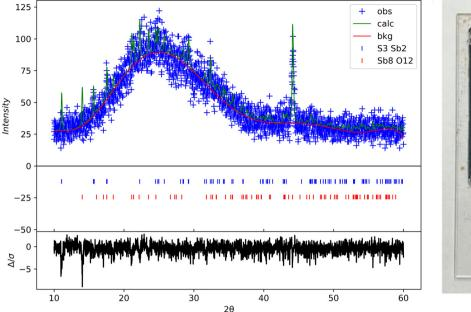
XRD scan of annealed Sb<sub>2</sub>S<sub>3</sub> thin films at 300 °C for 60 min on glass substrate. GSAS 2 refined XRD data (left); photo image of annealed sample (right).
