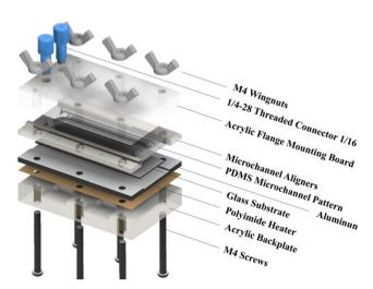
Fig. 1 Exploded view of MASL reactor.
