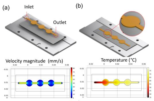
Fig. 4 COMSOL simulation results for reaction inlet velocity of 14.9 mm s<sup>-1</sup> at 20 °C on an 80 °C heating plate: (a) the velocity profile at center line, (b) the surface temperature.
