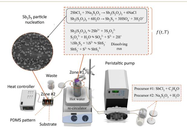
Fig. 2 Process schematics for Sb<sub>2</sub>S<sub>3</sub> thin films.
