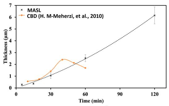
Fig. 9 Thickness vs. time comparison of MASL (this study) and chemical bath deposition.<sup>39</sup>
