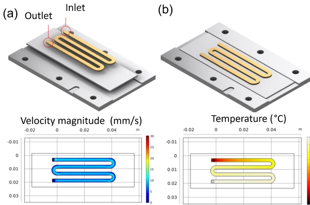
Fig. 3 COMSOL simulation results for reaction inlet velocity of  $14.9 \text{ mm s}^{-1}$  at  $35 \text{ }^\circ\text{C}$  on an  $80 \text{ }^\circ\text{C}$  heating plate: (a) the velocity profile at center line, (b) the surface temperature.
