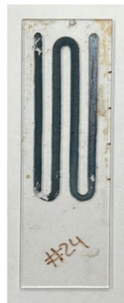
Fig. 10 XRD scan of annealed \text{Sb}_2\text{S}_3 thin films at 300\text{ }^\circ\text{C} for 60 min on glass substrate. GSAS 2 refined XRD data (left); photo image of annealed sample (right).
