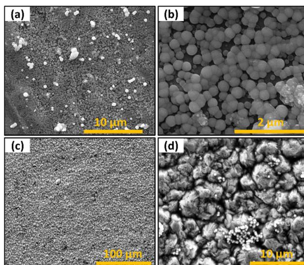
Fig. 12 SEM images of films deposited on current collector substrates (a)  $\text{Sb}_2\text{S}_3$  on Al substrate (b) higher magnification of  $\text{Sb}_2\text{S}_3$  on Al substrate (c)  $\text{Sb}_2\text{S}_3$  on Cu substrate (d) higher magnification of  $\text{Sb}_2\text{S}_3$  on Cu substrate.
