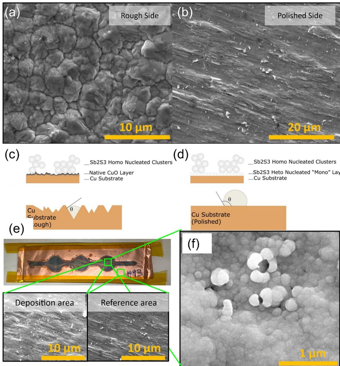
Fig. 13 SEM images of uncoated MTI Cu foil and nucleation barrier theory diagrams. (a) Rough side, (b) polished side, (c) native oxide barrier to heterogeneous nucleation, (d) removed native oxide nucleation, (e) optical image of the deposited film on polished and cleaned Cu foil and SEM images of deposited and non-deposited areas, (f)  $\text{Sb}_2\text{S}_3$  film deposited on polished copper foil substrates followed by HCl cleaning.
