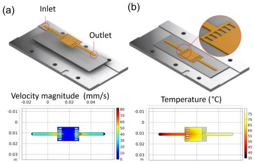
Fig. 5 COMSOL simulation results for reaction inlet velocity of 44 mm s<sup>-1</sup> at 40  $^{\circ}$ C on a 90  $^{\circ}$ C heating plate: (a) the velocity profile at the center line, (b) the surface temperature.
