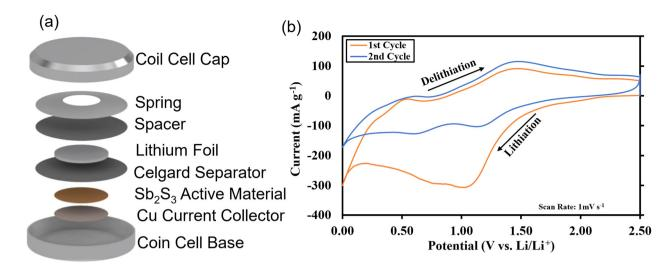
Fig. 14 Coin cell prototype schematic. (a) CAD model breakdown; (b) 1st and 2nd cycle cyclic voltammetry curves.
