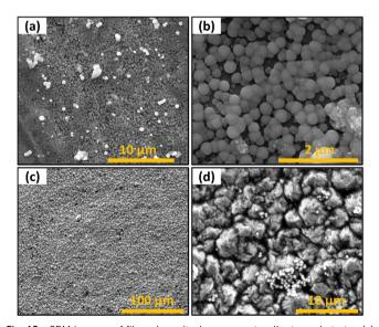
Fig. 12 SEM images of films deposited on current collector substrates (a)  $Sb_2S_3$  on Al substrate (b) higher magnification of  $Sb_2S_3$  on Al substrate (c) Sb<sub>2</sub>S<sub>3</sub> on Cu substrate (d) higher magnification of Sb<sub>2</sub>S<sub>3</sub> on Cu substrate.
