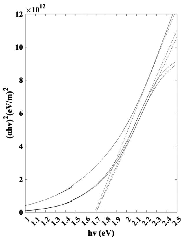
Fig. 11 Tauc plot for band gap calculation.
