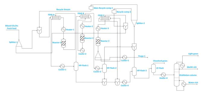
Fig. 4 Illustration of flowsheet 7B. This flowsheet features three reactors in series with intermediate cooling. This features a different feed, productpurge arrangement to the third reactor (reactor 3)
