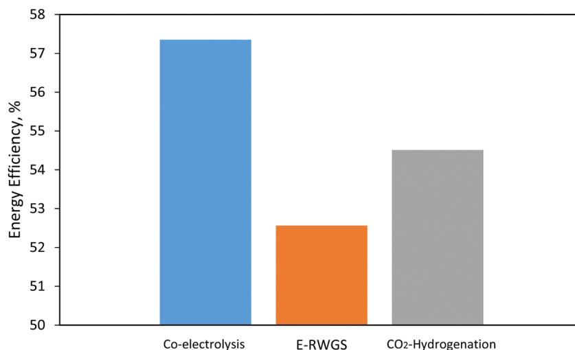
Fig. 13 Energy efficiency comparison of co-electrolysis, e-RWGS, and CO<sub>2</sub> based power to methanol process.
