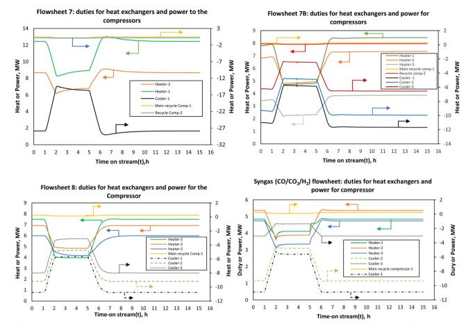
The heat duties and power of the compressors to the reactors when the load was changed from full (100%) to half-load (50%)
