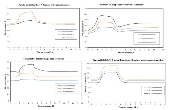
Fig. 12 The single pass reactor conversion for the three system configurations when the load was changed from full (105%) to half-load (50%).
