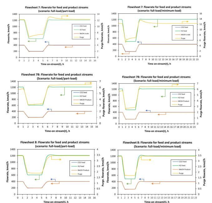
Fig. 7 Flowrate of the feed and the product streams when the load was changed from full-load (100%) to part-load (50%) and minimum load (40%). These results are for flowsheet 7, flowsheet 7B and flowsheet 8.
