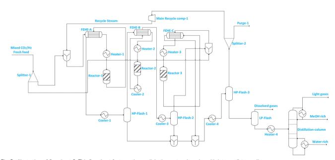
Fig. 5 Illustration of flowsheet 8. This flowsheet features three adiabatic reactors in series with intermediate cooling
