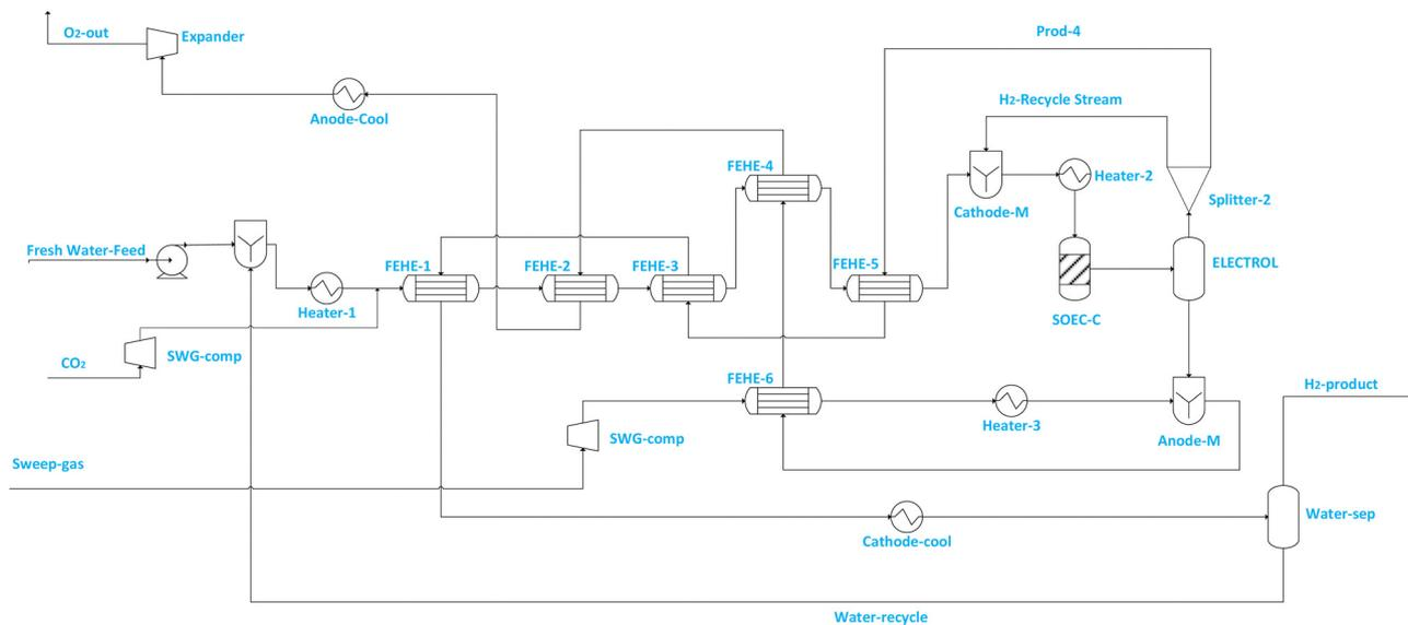
Fig. 2 Illustration of the SOEC unit used for co-electrolysis in ASPEN PLUS<sup>®</sup>.
