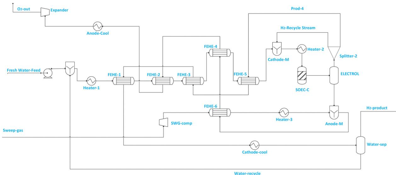
Fig. 1 Illustration of the SOEC unit used for steam electrolysis in ASPEN PLUS<sup>®</sup>.
