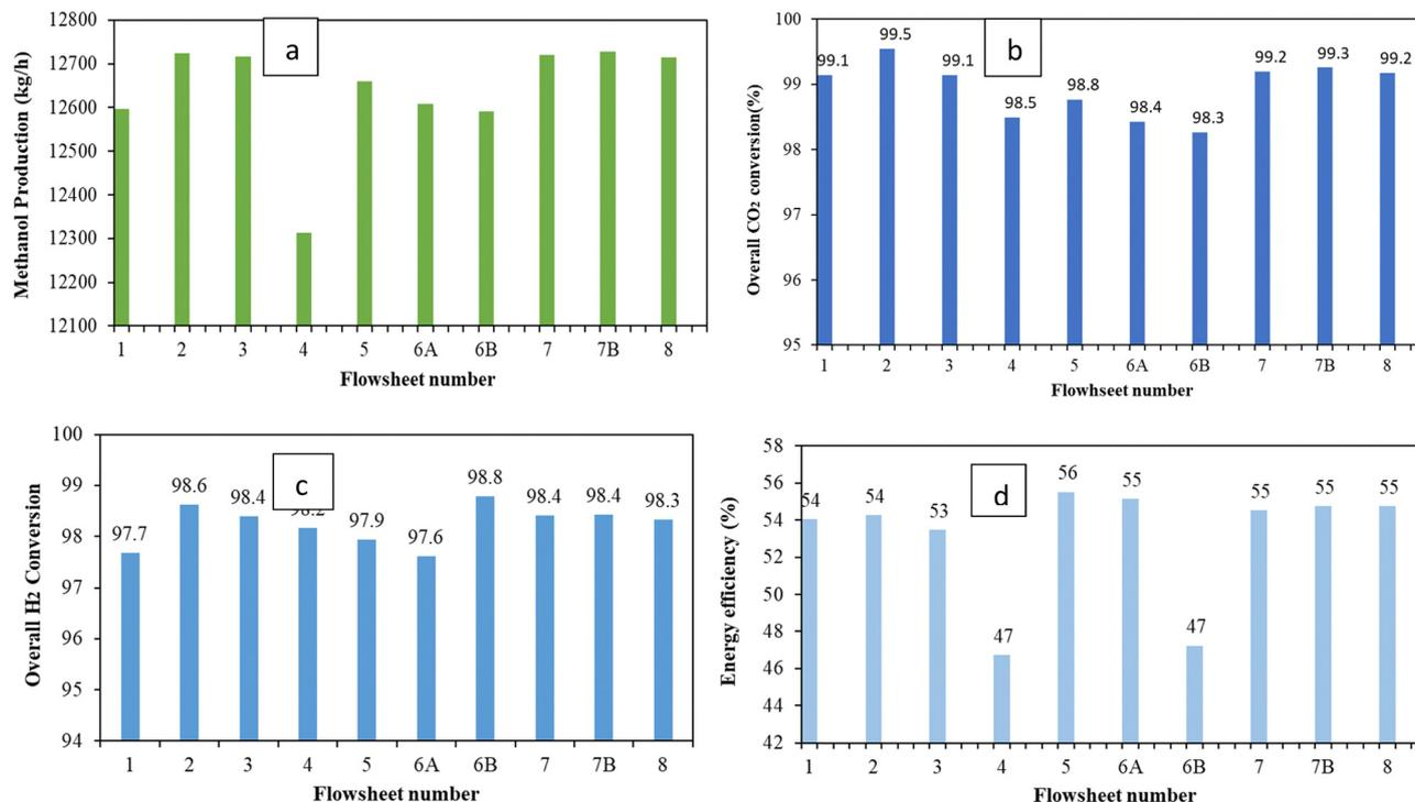
Fig. 6 Performance of the different flowsheets considered in this paper: (a) methanol production, (b) Overall CO<sub>2</sub> conversion, (c) overall H<sub>2</sub> conversion and (d) overall energy efficiency of the process.
