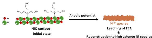
Fig. 5 Proposed transformation of the electrode surface of Ni/CP-TEA during the OER.
