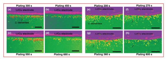
Fig. 13 Operando SEM images of the Li/Cu anode used by Rong et al. at increasing plating times for a solution containing (a)–(d)  $0.2 \text{ M Li}_2\text{S}_8$  and (e)–(h)  $0.2 \text{ M Li}_2\text{S}_8$  with 1 wt% LiNO<sub>3</sub>. Scale bar: 10  $\mu$ m ((a)–(h) adapted with permission from ref. 135, Copyright (2017) Wiley-VCH.)
