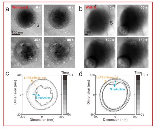
Fig. 14 (a) and (b) TEM image of sulfur nanoparticles during lithiation (a) without an ionic liquid electrolyte and (b) with ionic liquid electrolyte; (c) and (d) outer boundaries of sulfur particle and LiPS and their evolution over time from (a) and (b) respectively. ((a) – (d) Reproduced with permission from ref. 140, Copyright (2020) American Chemical Society.)
