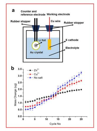
Fig. 15 (a) Schematic of an EQCM set-up for an LSB; (b) mass change measured through EQCM for the lithium anode with an electrolyte containing either no salt (blue) or TMA salt (Zn<sup>2+</sup> in black and Cu<sup>2+</sup> in red). ((a) and (b) Reproduced with permission from ref. 146, Copyright (2019) Elsevier.)
