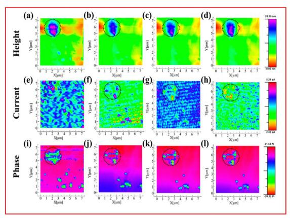
Fig. 12 AFM-SECM images of insoluble  $\text{Li}_2\text{S/Li}_2\text{S}_2$  on the cathode. Simultaneously obtained data for the height (a)–(d), current (e)–(h) and phase shift (i)–(l) mapping are shown for samples before oxidation (a), (e), (i), at 2.5 V (b), (f), (j), 2.6 V (c), (g), (k) and 2.7 V (d), (h), (l) vs.  $\text{Li/Li}^+$ . ((a)–(l) Reproduced with permission from ref. 132, Copyright (2019) American Chemical Society.)
