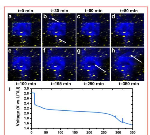
Fig. 10 (a)—(h) XRF map of a LSB with sulfur (blue) and cobalt (yellow) following changes in voltage corresponding with (i) a discharge voltage profile. (a)—(i) Reproduced with permission from ref. 86, Copyright (2022) American Chemical Society.
