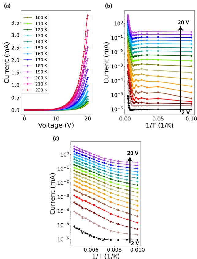
Fig. 4 (a)  $I$ - $V$  relationship of a  $200 \times 200 \mu\text{m}^2$  device from sample 2 from 100 K to 220 K in steps of 10 K. (b) Semi-log plot of  $I - 1/T$  from 2 V to 20 V in steps of 1 V. (c) Semi-log plot of  $I - 1/T$  from 2 V to 20 V in steps of 1 V and the fitting of the  $I - 1/T$  relationship.
