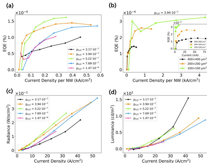
**Fig. 3** (a) EQE vs.  $J$  of samples 1–5 with an active region area of  $400 \times 400 \mu\text{m}^2$ . (b) EQE vs.  $J$  of sample 2 with varying active region area. The inset shows the EQE vs. applied current for the same devices. (c) Radiance vs.  $J$  of samples 1–5 with an active region area of  $400 \times 400 \mu\text{m}^2$ . (d) Luminance vs.  $J$  of samples 1–5 with an active region area of  $400 \times 400 \mu\text{m}^2$ .
