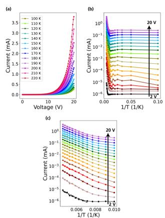
Fig. 4 (a) I-V relationship of a 200  $\times$  200  $\mu m^2$  device from sample 2 from 100 K to 220 K in steps of 10 K. (b) Semi-log plot of I - 1/T from 2 V to 20 V in steps of 1 V. (c) Semi-log plot of I - 1/T from 2 V to 20 V in steps of 1 V and the fitting of the I - 1/T relationship.
