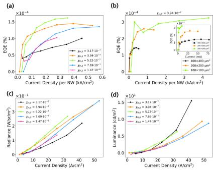
Fig. 3 (a) EQE vs. J of samples 1–5 with an active region area of  $400 \times 400 \,\mu\text{m}^2$ . (b) EQE vs. J of sample 2 with varying active region area. The inset shows the EQE vs. applied current for the same devices. (c) Radiance vs. J of samples 1-5 with an active region area of  $400 \times 400 \, \mu m^2$ . (d) Luminance vs. J of samples 1–5 with an active region area of  $400 \times 400 \, \mu m^2$
