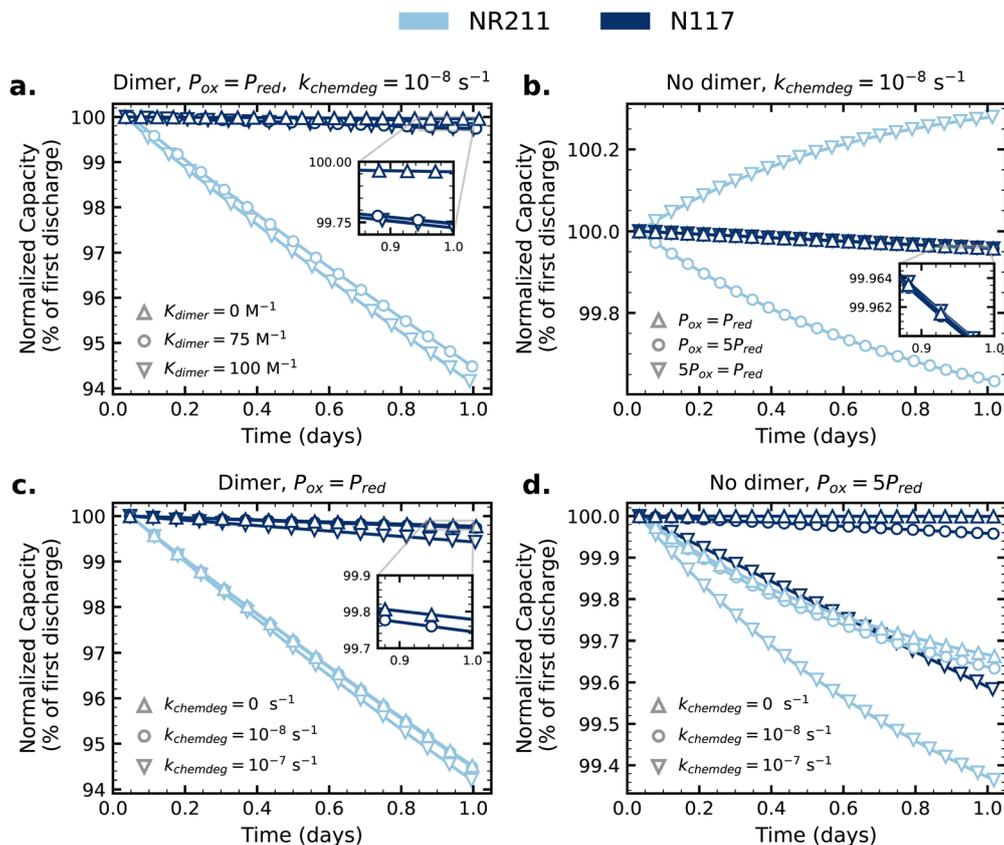
**Fig. 5** Simulated cycling of symmetric cells with parameters varied to explore other possible modes of net crossover (parameters and resulting capacity fade rates listed in Table S3, non-normalized capacity in Fig. S12, ESI†). In (a) and (b), “NR211” and “N117” traces with  $K_{\text{dimer}} = 0$  overlap completely. Model parameters are tabulated in Table S3 (ESI†), with membrane permeabilities based on experimental values for pretreated membranes.
