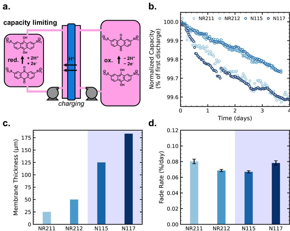
**Fig. 1** (a) Schematic of the AQDS symmetric cell depicted in charging mode; (b) discharge capacity over time for symmetric cells with as-received membranes, normalized by the capacity of the first discharge; (c) nominal membrane thicknesses; and (d) capacity fade rates for cells with each Nafion membrane (as-received), with error bars denoting uncertainty in a given single-cell fade rate measurement as per ref. 24.
