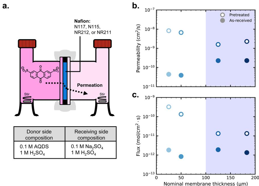
**Fig. 2** (a) Schematic H-cell for permeability measurements and compositions of donating and receiving chambers; (b) permeabilities of as-received and pretreated Nafion membranes; (c) diffusion-driven crossover fluxes of AQDS for each membrane based on the permeability measurements.
