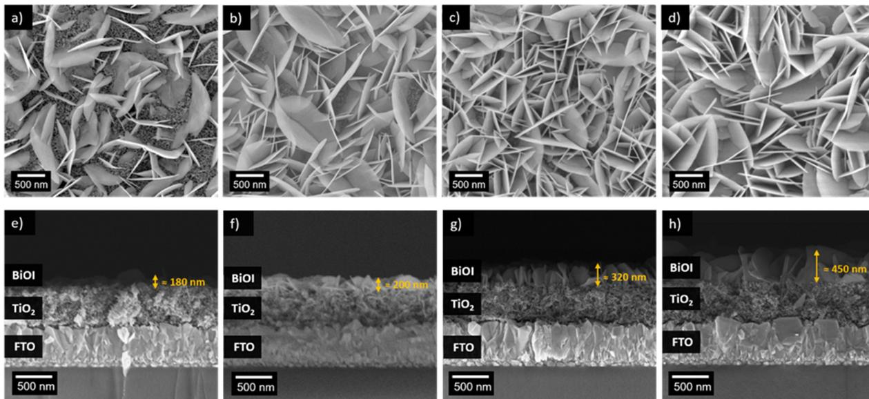
Fig. 3 SEM images of T/BiOI films obtained by Autodrop with different dropping volumes in top-view and cross-section: (a) and (e) T/BiOI 0.4; (b) and (f) T/BiOI 0.8; (c) and (g) T/BiOI 1.2; (d) and (h) T/BiOI 1.6.
