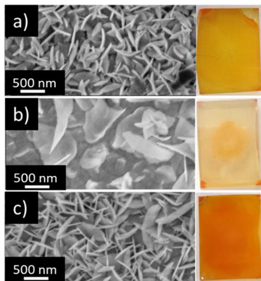
Fig. 2 SEM images (left) and respective macroscopic photos (right) of large area BiOI thin films ( $1 \times 2 \text{ cm}^2$ ) prepared by the AutoDrop method on top of (a) FTO glass, (b) FTO-planar  $\text{TiO}_2$ , (c) FTO-mesoporous  $\text{TiO}_2$ .
