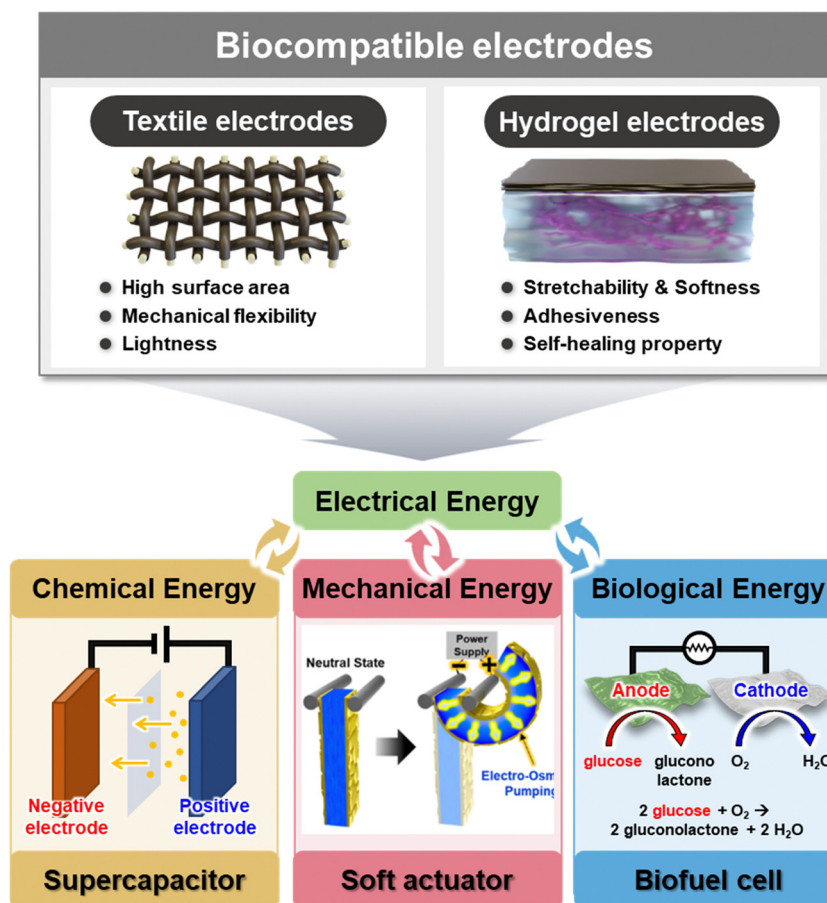
Fig. 1 Schematic illustration of textile-based and hydrogel-based biocompatible electrodes for the application of various energy storage and conversion devices, such as supercapacitor, biofuel cell, and soft actuator.
