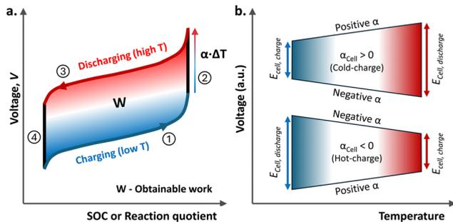
Fig. 1 (a) Voltage–SOC diagram of TREC for  $\alpha_{\text{Cell}} > 0$  with its sequence of operation (#1 to #4) and (b) open circuit voltage shifts by electrolyte temperature change for both positive (upper) and negative  $\alpha_{\text{Cell}}$  cases (lower).
