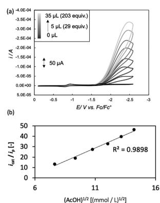
Fig. 5 (a) CVs and (b) plots of  $i_{\rm cat}/i_{\rm p}$  A vs. (AcOH) $^{1/2}$ /(mmol L $^{-1}$ ) $^{1/2}$  of complex 1 (1.0 mM) in the presence of 0-203 equiv. of AcOH (p $K_a$  = 22.3 in MeCN) in MeCN containing 0.1 M TBAP at room temperature under an Ar atmosphere, recorded at a scan rate of 500 mV s<sup>-1</sup>.
