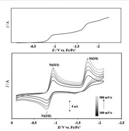
Fig. 3 Cyclic voltammograms (bottom) of complex  ${\bf 1}$  in MeCN, as measured at several sweep rates and current integral (upper) estimated by DPV. Note that the redox potential of ligand  $L_H$  may be observed in this region, but as shown in Fig. S6 of ESI,† no such wave was detected when the CV measurement of ligand  $L_H$  was carried out under the same conditions as complex  ${\bf 1}$ , and the wave is due to the Ni(I/O) couple of complex  ${\bf 1}$ .
