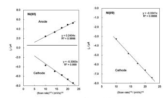
Fig. 4 Plots of  $i_p/\mu A$  vs. (scan rate)<sup>1/2</sup>/(mV s<sup>-1</sup>)<sup>1/2</sup> of Ni(II/I) (left) and Ni(I/O) (right) of complex **1** in MeCN.
