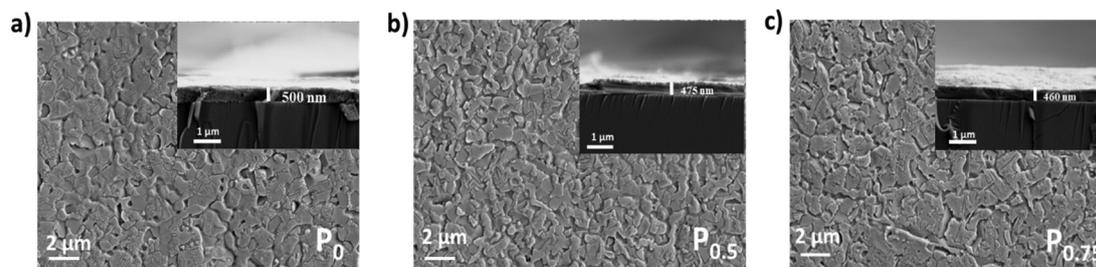
**Fig. 2** Surface and cross-sectional images (given in the inset) of (a)  $P_0$ , (b)  $P_{0.5}$ , and (c)  $P_{0.75}$  compositions. [ $P_0$  = pristine  $(\text{PEA})_2\text{PbI}_4$ ,  $P_{0.5}$  = 0.5 mg PCBM mixed in 1 ml  $(\text{PEA})_2\text{PbI}_4$  perovskite precursor, and  $P_{0.75}$  = 0.75 mg PCBM mixed in 1 ml  $(\text{PEA})_2\text{PbI}_4$  perovskite precursor solution.]
