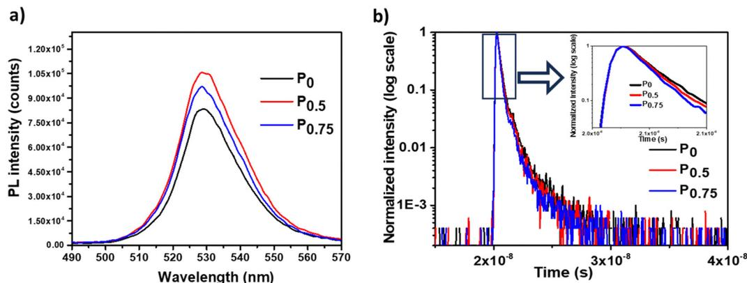
Fig. 3 (a) SSPL and (b) TRPL curves of  $P_0$ ,  $P_{0.5}$  and  $P_{0.75}$  compositions. [ $P_0$  = pristine  $(\text{PEA})_2\text{PbI}_4$ ,  $P_{0.5}$  = 0.5 mg PCBM mixed in 1 ml  $(\text{PEA})_2\text{PbI}_4$  perovskite precursor, and  $P_{0.75}$  = 0.75 mg PCBM mixed in 1 ml  $(\text{PEA})_2\text{PbI}_4$  perovskite precursor solution].
