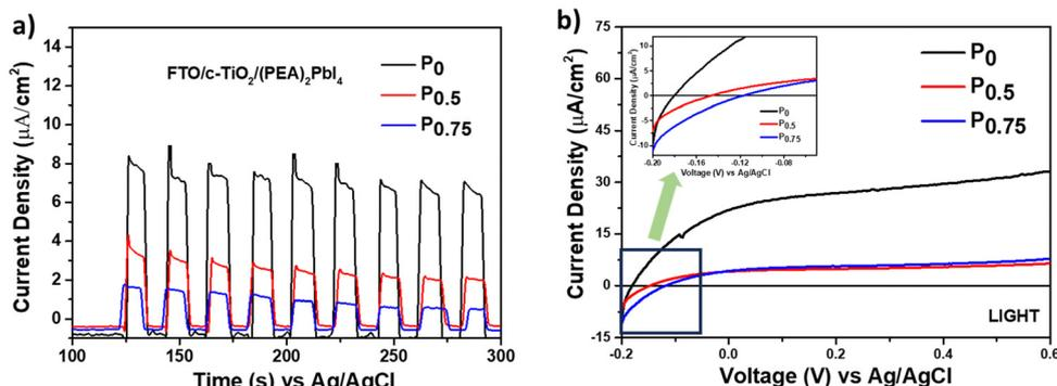
Fig. 4 (a) The chronoamperometric and (b) LSV curves (over c-TiO<sub>2</sub>) of P<sub>0</sub>, P<sub>0.5</sub>, and P<sub>0.75</sub> compositions. [P<sub>0</sub> = pristine (PEA)<sub>2</sub>PbI<sub>4</sub>, P<sub>0.5</sub> = 0.5 mg PCBM mixed in 1 ml (PEA)<sub>2</sub>PbI<sub>4</sub> perovskite precursor, and P<sub>0.75</sub> = 0.75 mg PCBM mixed in 1 ml (PEA)<sub>2</sub>PbI<sub>4</sub> perovskite precursor solution.]
