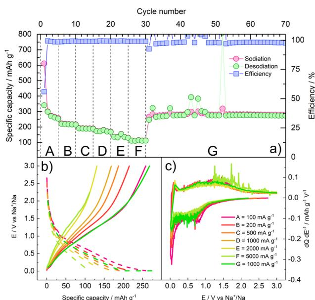
**Fig. 5** Rate capability of  $\gamma\text{-Fe}_2\text{O}_3/\text{rGO}$ . (a) cycle number vs. specific capacity/efficiency; (b) galvanostatic  $E$  vs.  $Q$  profiles at each current value; (c) differential  $E$  vs.  $dQ/dE^{-1}$  profiles at each current value. The current values applied at each step are detailed in Table 1.
