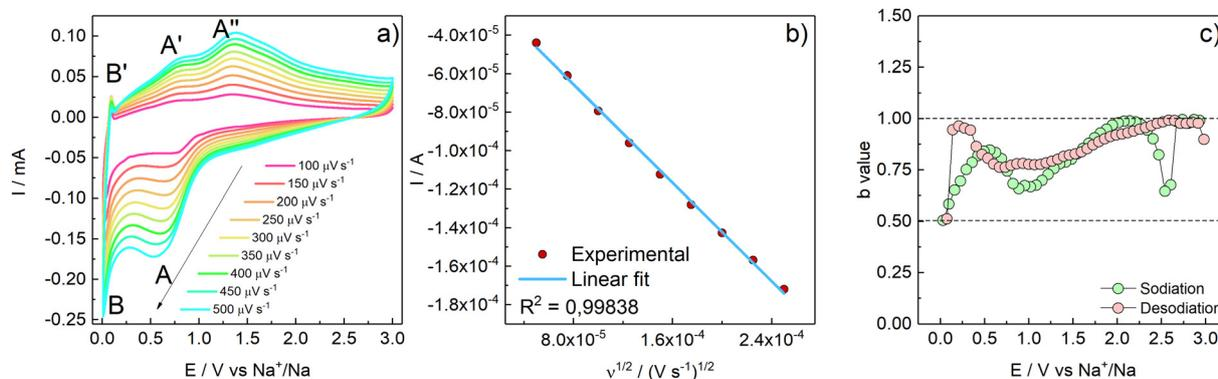
Fig. 6 (a) Cyclic voltammograms acquired at different scan rates from 100 up to 500  $\mu\text{V s}^{-1}$  (50  $\mu\text{V s}^{-1}$  increment steps). (b)  $I$  vs.  $\nu^{1/2}$  plot with linear fit of peak A. (c) calculated  $b$ -values vs.  $E$ .
