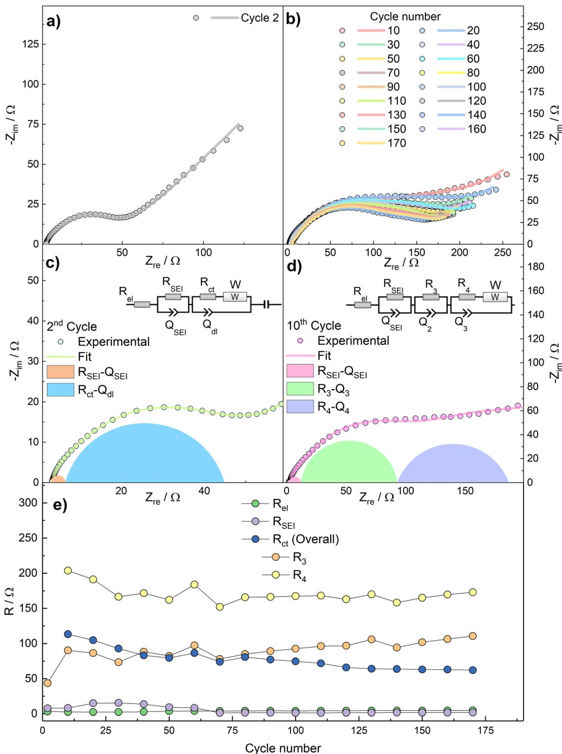
Fig. 7 Nyquist plot as well as fit of (a) 2<sup>nd</sup> cycle and (b) from 10<sup>th</sup> cycle onwards. Panel (c) and (d) graphic demonstration of the fit of the 2<sup>nd</sup> and 10<sup>th</sup> cycles, respectively. (e) Fit results obtained by using the equivalent circuit models in panels (c) and (d).
