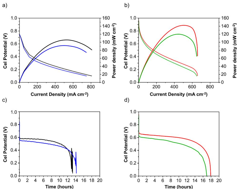
Fig. 5 Direct formate fuel cell experiments containing the Pd/C (a) and (c) and PdAu/C anode (b) and (d). All cells used FeCo/C cathode catalyst and Fumatech FAA-3-30 AEM. The fuel was 1 M HCOOK and 1 M KOH.  $T_{cell}$  60 °C: figures (a) and (b) are voltage and power density curves. Figures (c) and (d) are cell voltage at constant current density 0.05 A cm<sup>-2</sup>. First and fifth cycle for Pd/C are respectively black and blue curves, while for PdAu/C are red and green.
