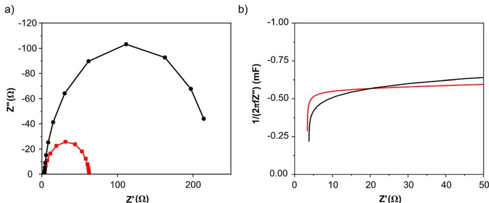
Fig. 4 Electrochemical impedance spectroscopy (EIS) of PdAu/C (red curves) and Pd/C (black curves) in KOH 2 M at 0.4 V vs. RHE: (a) Nyquist plot and (b) capacitance plot.
