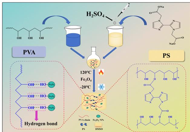
Fig. 1 Schematic diagram of the preparation of the PVA/PS/Fe<sub>3</sub>O<sub>4</sub> organogel.
