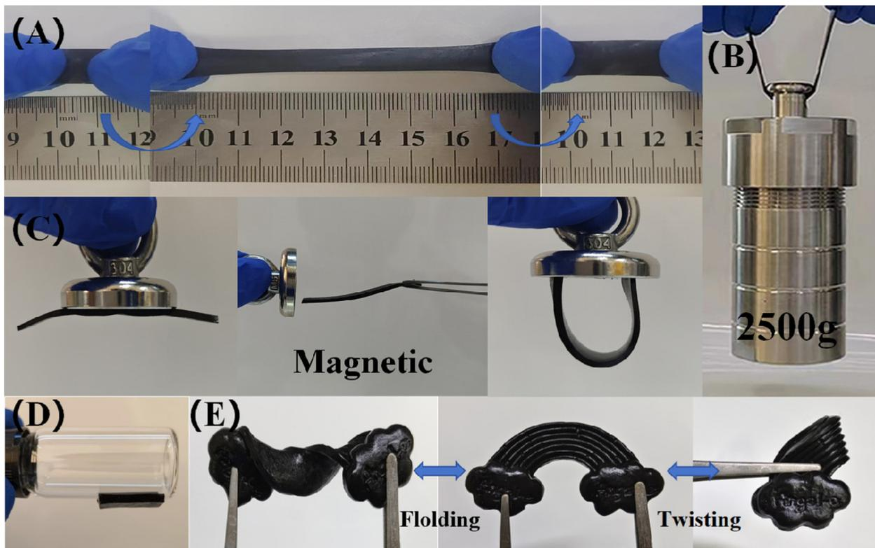
**Fig. 3** (A) and (B) PVA/PS/Fe<sub>3</sub>O<sub>4</sub> organogel exhibiting load-bearing capability and stretchability. (C) Magnetic response of the organogel under the action of magnets. (D) Adhesion of the organogel. (E) Deformation performance of the as-prepared organogel.
