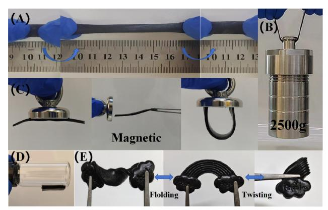
Fig. 3 (A) and (B) PVA/PS/Fe<sub>x</sub>O<sub>4</sub> organogel exhibiting load-bearing capability and stretchability. (C) Magnetic response of the organogel under the action of magnets. (D) Adhesion of the organogel. (E) Deformation performance of the as-prepared organogel.
