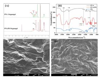
**Fig. 2** (A) <sup>1</sup>H nuclear magnetic resonance (NMR) spectra of the samples. (B) Fourier transform infrared (FT-IR) spectra of the samples. (C) Scanning electron microscopy image of the PVA organogel. (D) Scanning electron microscopy image of the PVA/PS organogel.
