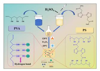
Fig. 1 Schematic diagram of the preparation of the PVA/PS/Fe $_3\mathrm{O}_4$  organogel.
