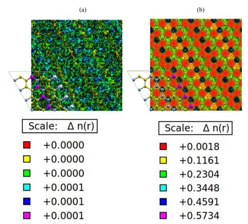
Fig. 6 (a) AlN:CC:GaN:CC, (b) AlN:CC:BN:CC isoline–isosurface charge density. Violet depicts regions of maximum charge density. Red depicts regions of minimum density in charge.
