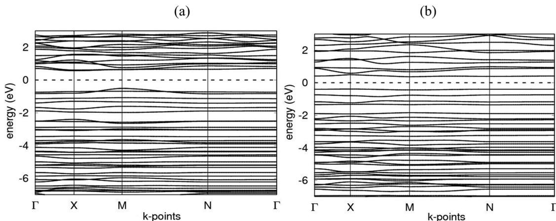
Fig. 2 Computed band structures in the  $\Gamma$ -X-M-N- $\Gamma$  direction for (a) nanoarchitecture-A, and (b) nanoarchitecture-B. The zero of the energy scale is set at the middle of the energy gap,  $E_g$ , between the valence and conduction bands.
