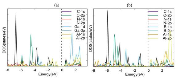
Fig. 4 Partial density of states (p-DOS) diagrams for (a) AIN:CC:GaN:CC & (b) AIN:CC:BN:CC modes.
