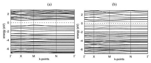
Fig. 2 Computed band structures in the  $\Gamma - X - M - N - \Gamma$  direction for (a) nanoarchitecture-A, and (b) nanoarchitecture-B. The zero of the energy scale is set at the middle of the energy gap,  $E_{\rm g}$ , between the valence and conduction bands.
