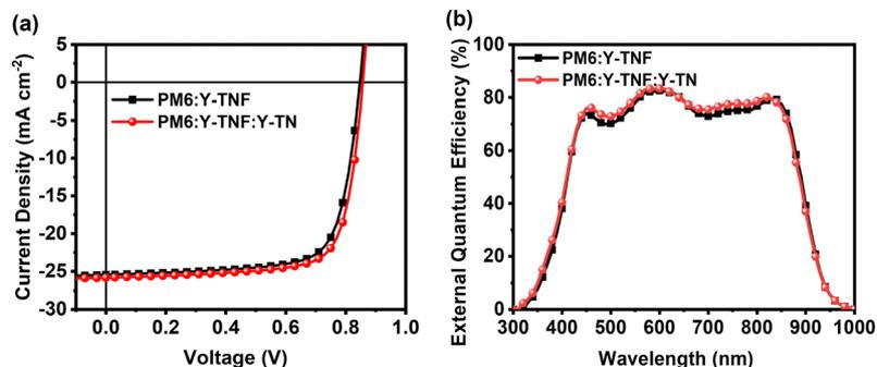
Fig. 3 (a)  $J$ - $V$  plots of the PM6:Y-TNF:Y-TN-based OSCs (1:1:0 and 1:1:0.1, w/w/w) with 0.25% DIO additive, and a TA treatment at  $100 \text{ }^\circ\text{C}$  for 5 min under an illumination of AM 1.5 G,  $100 \text{ mW cm}^{-2}$ , and (b) EQE curves of the corresponding OSCs.
