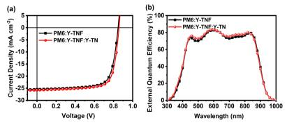
Fig. 3 (a) J-V plots of the PM6: Y-TNF: Y-TN-based OSCs (1:1:0 and 1:1:0.1, w/w/w) with 0.25% DIO additive, and a TA treatment at 100 °C for 5 min under an illumination of AM 1.5 G, 100 mW cm<sup>-2</sup>, and (b) EQE curves of the corresponding OSCs.
