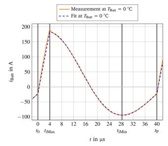
Fig. 3 Measured and fitted current  $i_{Batt}$  for one period at a battery temperature of  $T_{\text{Batt}} = 0 \, ^{\circ}\text{C}$ .
