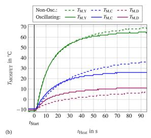
Fig. 2 Comparison of the oscillating and non-oscillating circuits. In (a) the current and voltage waveforms during a switching period and in (b) the temperature rise of the three MOSFETs during the first 90 s.
