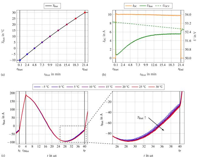
Fig. 4 Summary of the whole heating process at  $T_{Amb}$  = 10 K, stopping the heating at  $T_{Batt}$  = 30 K. (a) The temperature  $T_{Batt}$  (b) the current  $I_{Batt}$  and the voltage  $U_{Batt}$  with the calculated open circuit voltage  $U_{OCV}$  (c) the current waveform  $I_{Batt}$  for one switching period for each temperature increment of 5 K of  $T_{Batt}$ .
