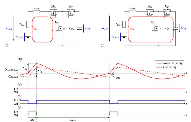
Fig. 1 Equivalent circuit diagram of the heater showing the current flow during the short sequence in (a) and the oscillating sequence in (b),  $Z_{\text{Batt}}$  and  $U_{\text{OCV}}$  representing the whole battery. (c) Displays the idealized current waveforms for the non-oscillating and oscillating heater, as well as the switching states of the MOSFETs for both approaches. The implemented dead time is not depicted.
