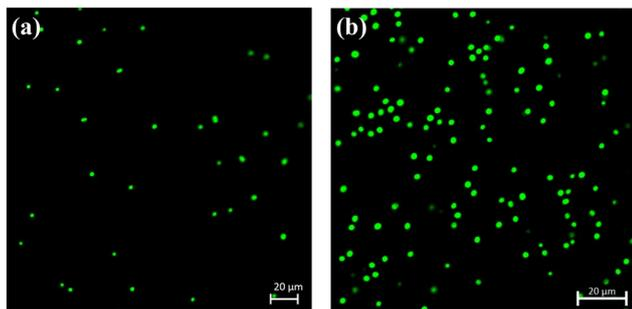
Fig. 9 Results of confocal microscopy analysis for (a) *Synechocystis* sp. PCC 6803 culture, scale bar -20  $\mu\text{m}$ . (b) *Synechocystis* sp. PCC 6803 seeded 3D bio-anode structure, scale bar -20  $\mu\text{m}$ .
