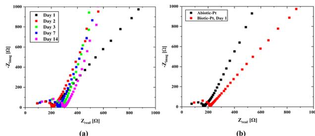
**Fig. 7** EIS results of biotic and abiotic systems in the range of 1 MHz to 100 Hz with 10 mV signal amplitude. (a) Daily potentiostatic EIS results of the biotic scaffold with Pt/air cathode electrodes. (b) Potentiostatic EIS results of biotic and abiotic scaffolds with Pt/air cathode electrodes.
