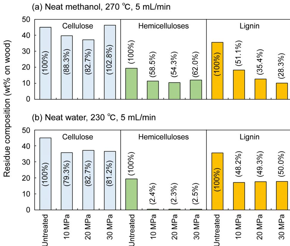
Fig. 4 Composition of the insoluble residue after the treatment of Japanese cedar wood with (a) neat methanol (from room temperature to 270 °C (8 °C min<sup>-1</sup>) and at 270 °C for 30 min) or (b) neat water (from room temperature to 230 °C (8 °C min<sup>-1</sup>) and at 230 °C for 30 min) at various pressures.
