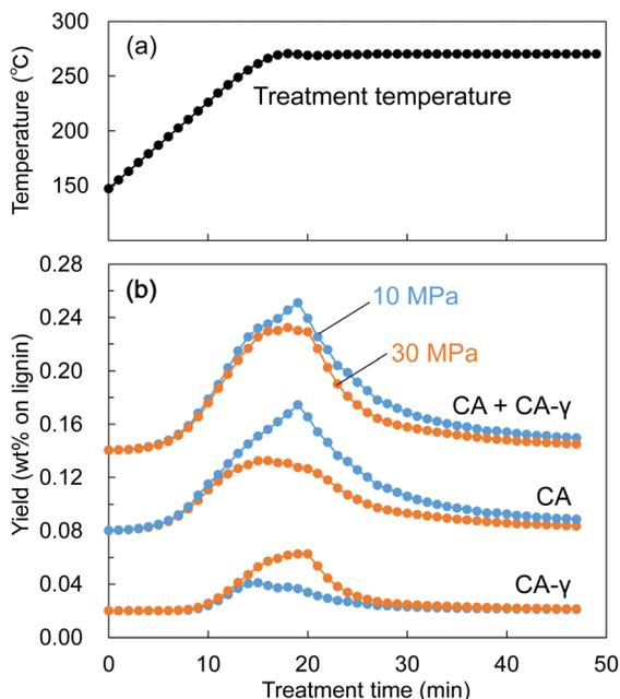
Fig. 10 Changes in (a) treatment temperature and (b) the yields of lignin-derived monomers during the treatment of Japanese cedar wood with methanol/water (90/10, v/v) at 10 or 30 MPa at a flow rate of 5 mL min<sup>-1</sup>.
