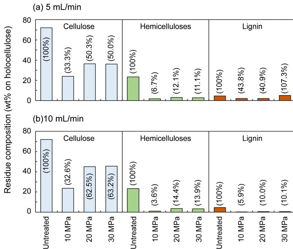
Fig. 3 Composition of the insoluble residue after the treatment of holocellulose with methanol/water (90/10, v/v) from room temperature to 270 °C (8 °C min<sup>-1</sup>) and at 270 °C for 30 min at various flow rates, (a) 5 mL min<sup>-1</sup>, and (b) 10 mL min<sup>-1</sup>, and pressures.
