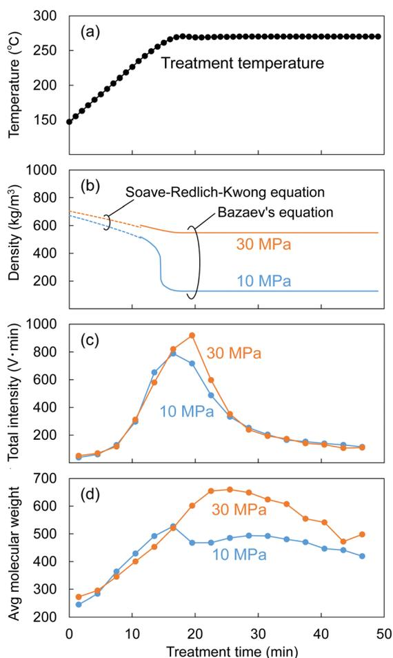
**Fig. 9** Changes in (a) treatment temperature, (b) density of methanol/water (90/10, v/v), (c) total intensity, and (d) average molecular weight of lignin-derived products estimated by gel permeation chromatography (GPC) analysis during the treatment of Japanese cedar wood with methanol/water at 10 or 30 MPa at a flow rate of 5 mL min<sup>-1</sup>.
