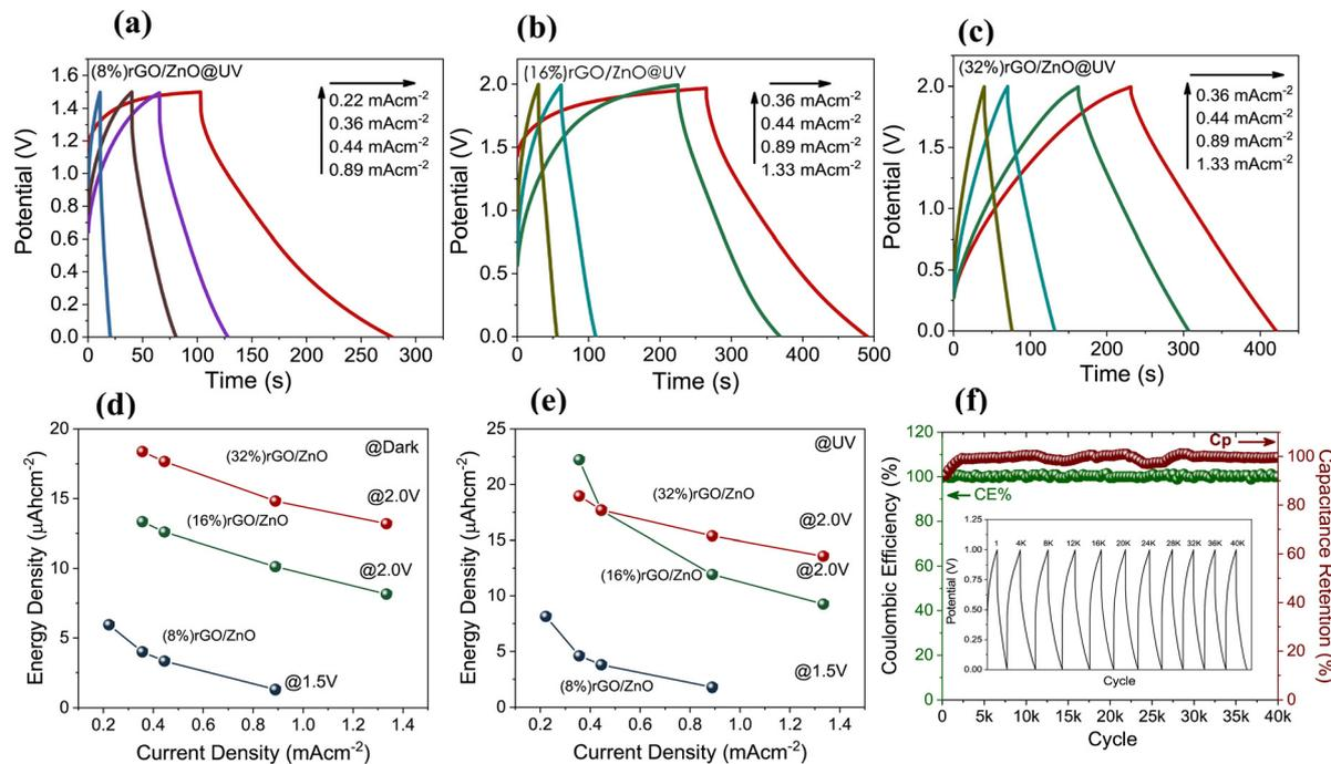
**Fig. 5** GCD curves of the (a) (8%) rGO/3D ZnO, (b) (16%) rGO/3D ZnO, and (c) (32%) rGO/3D ZnO under UV illumination (8.8 mW of power intensity), energy density values in the (d) dark and (e) UV illuminated environments, and (f) long term cycling stability of the PSC devices based on the (16%) rGO/3D ZnO composite material with the inset figure displaying the GCD curves at specific cycles.
