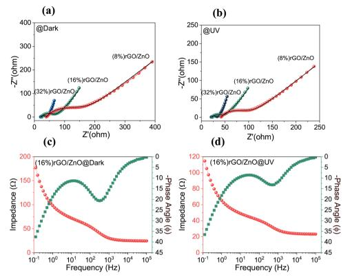
Fig. 7 Nyquist plots of rGO/3D ZnO photoelectrodes (a) in the dark and (b) under UV illumination, Bode plots of the (16%) rGO/3D ZnO based PSC device (c) in the dark and (d) under UV light.
