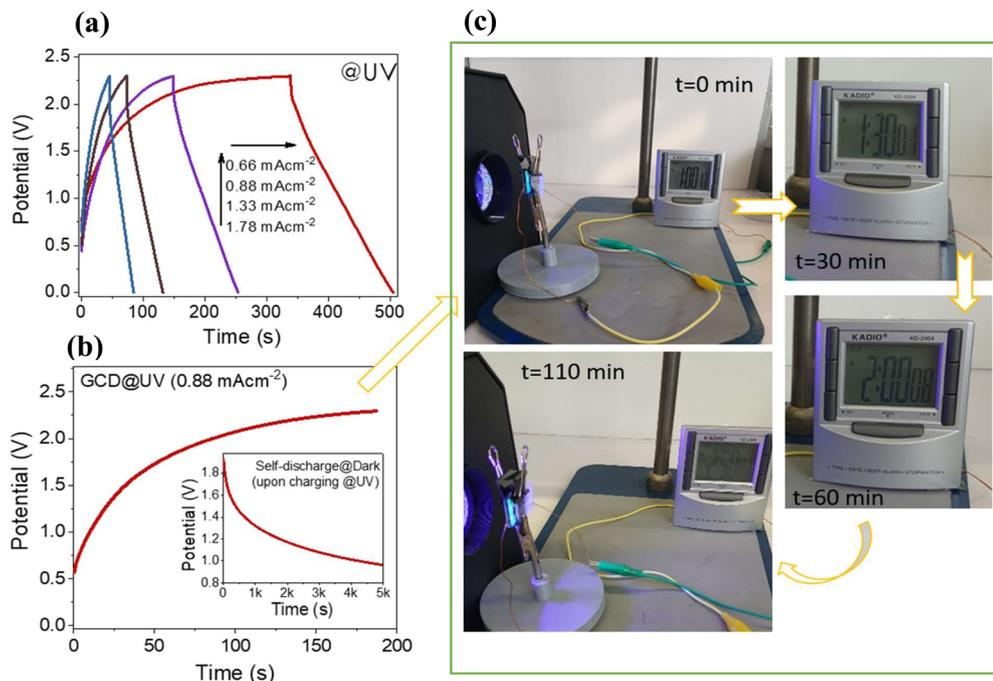
Fig. 8 Proof of concept experiments: (a) GCD curves at 2.2 V under UV illumination, (b) charging at a  $0.88 \text{ mA cm}^{-2}$  current density, and (c) photographic images of the PSC device for powering a digital watch after charging under UV illumination.
