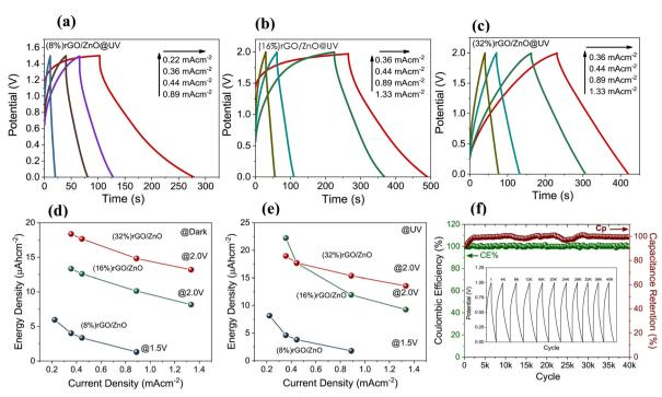
Fig. 5 GCD curves of the (a) (8%) rGO/3D ZnO, (b) (16%) rGO/3D ZnO, and (c) (32%) rGO/3D ZnO under UV illumination (8.8 mW of power intensity), energy density values in the (d) dark and (e) UV illuminated environments, and (f) long term cycling stability of the PSC devices based on the (16%) rGO/3D ZnO composite material with the inset figure displaying the GCD curves at specific cycles.
