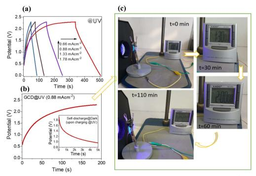
Fig. 8 Proof of concept experiments: (a) GCD curves at 2.2 V under UV illumination, (b) charging at a  $0.88 \text{ mA cm}^{-2}$  current density, and (c) photographic images of the PSC device for powering a digital watch after charging under UV illumination.
