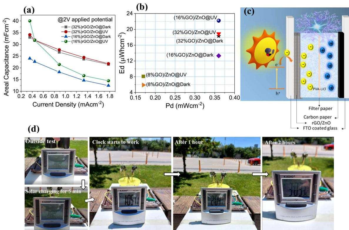
**Fig. 6** (a) Comparative areal capacitance values depending on the applied current density at a 2 V potential range, (b) Ragone plot and (c) schematic diagram of the photo charge–discharge step, and (d) pictures taken from the outdoor test.
