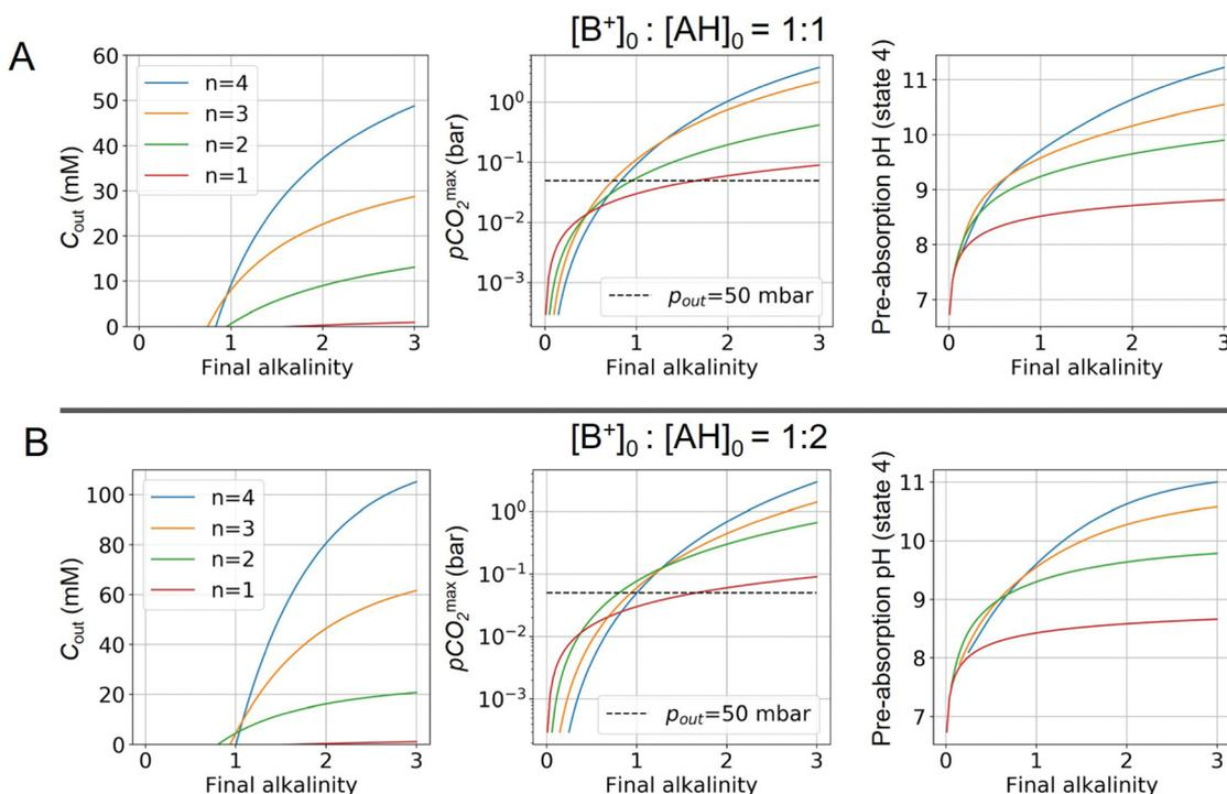
**Fig. 4** ABCS process output.  $C_{out}$  (left),  $p_{CO_2}^{max}$  (middle), and  $pH_4$  (right) are plotted as functions of final alkalinity. (A)  $[B^+] : [AH] = 1 : 1$ ; (B)  $[B^+] : [AH] = 1 : 2$ . Each reaction order is modelled with the corresponding optimal initial concentration and  $pK_{a,n}$ , taken from Fig. 3. For all points,  $p_{in} = 0.3$  mbar;  $p_{out}$  is chosen at 50 mbar and denoted with a black dashed line in the middle plots.
