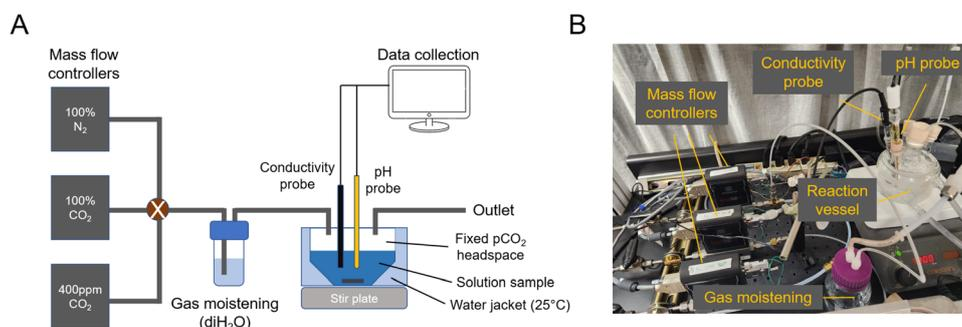
Fig. 5 Absorption and outgassing setup. (A) Schematic of mass flow controllers and reactor vessel. (B) Image of setup.
