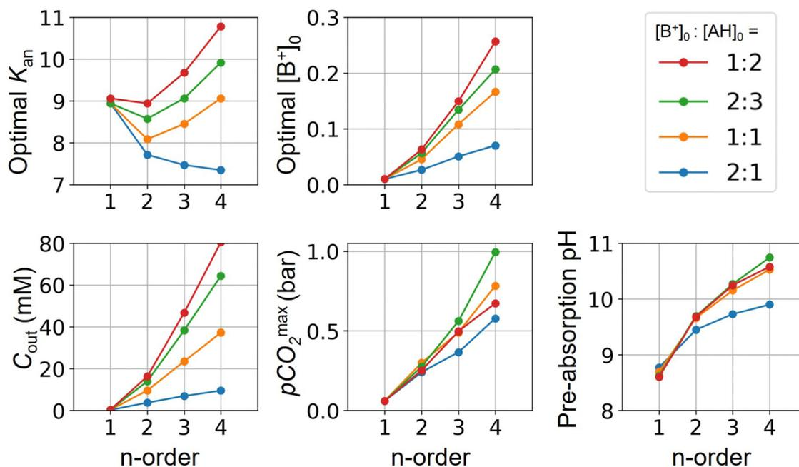
Fig. 3 ABCS optimization analysis. The optimal  $n$ th-order equilibrium constant ( $K_{a,n}$ ) and initial strong base concentrations ( $[B^+]_0$ ) are reported for each reaction order (1, 2, 3, and 4), and for four strong base (or alkalinity) to weak acid ratios: 2 : 1, 1 : 1, 2 : 3, and 1 : 2. The corresponding  $C_{\text{out}}$ ,  $p\text{CO}_2^{\text{max}}$ , and  $\text{pH}_4$ , at each optimal point is plotted. Each optimal point corresponds to the red dot in ESI,<sup>†</sup> Fig. C2.
