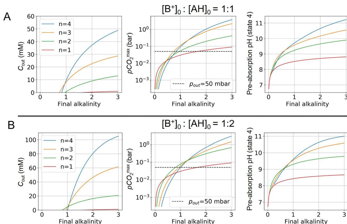
**Fig. 4** ABCS process output.  $C_{out}$  (left),  $p_{CO_2}^{max}$  (middle), and  $pH_4$  (right) are plotted as functions of final alkalinity. (A)  $[B^+]_0 : [AH]_0 = 1:1$ ; (B)  $[B^+]_0 : [AH]_0 = 1:2$ . Each reaction order is modelled with the corresponding optimal initial concentration and  $pK_{a,n}$ , taken from Fig. 3. For all points,  $p_{in} = 0.3$  mbar;  $p_{out}$  is chosen at 50 mbar and denoted with a black dashed line in the middle plots.
