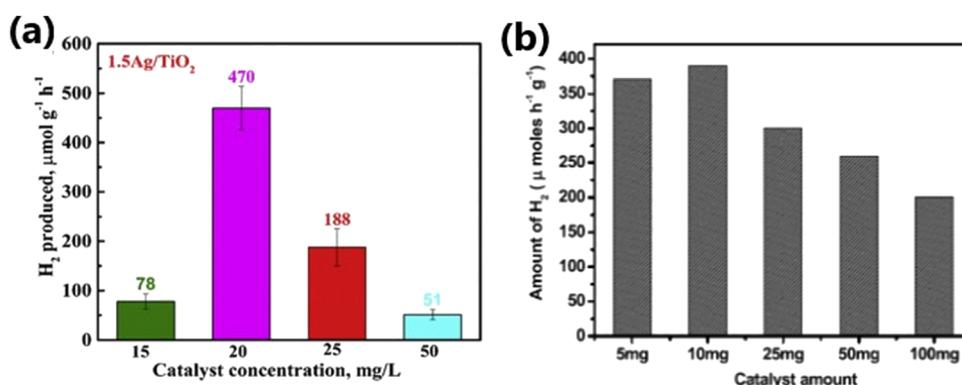
Fig. 25 (a) Photocatalytic hydrogen evolution activity of Ag/TiO<sub>2</sub> by varying the amount of catalyst. Reproduced with permission from ref. 112. Copyright ©2019, Elsevier Ltd. (b) Variation in photocatalytic H<sub>2</sub> evolution rate with respect to the amount of Ni/ $\gamma$ -Al<sub>2</sub>O<sub>3</sub>/CNT-TiO<sub>2</sub> catalyst. Reproduced with permission from ref. 102. Copyright ©2017, Elsevier Ltd.
