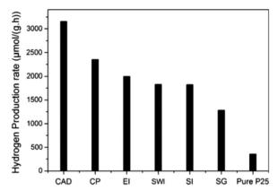
Fig. 17 Comparison of the photocatalytic hydrogen evolution rate on pure P25 and  $\text{CuO/TiO}_2$  samples produced by different preparation methods, namely chemical adsorption decomposition (CAD), composite precipitation (CP), ethanol impregnation (EI), simple wet impregnation (SWI), stepwise impregnation (SI), and sol-gel (SG). Reproduced with permission from ref. 184. Copyright ©2014, Springer.
