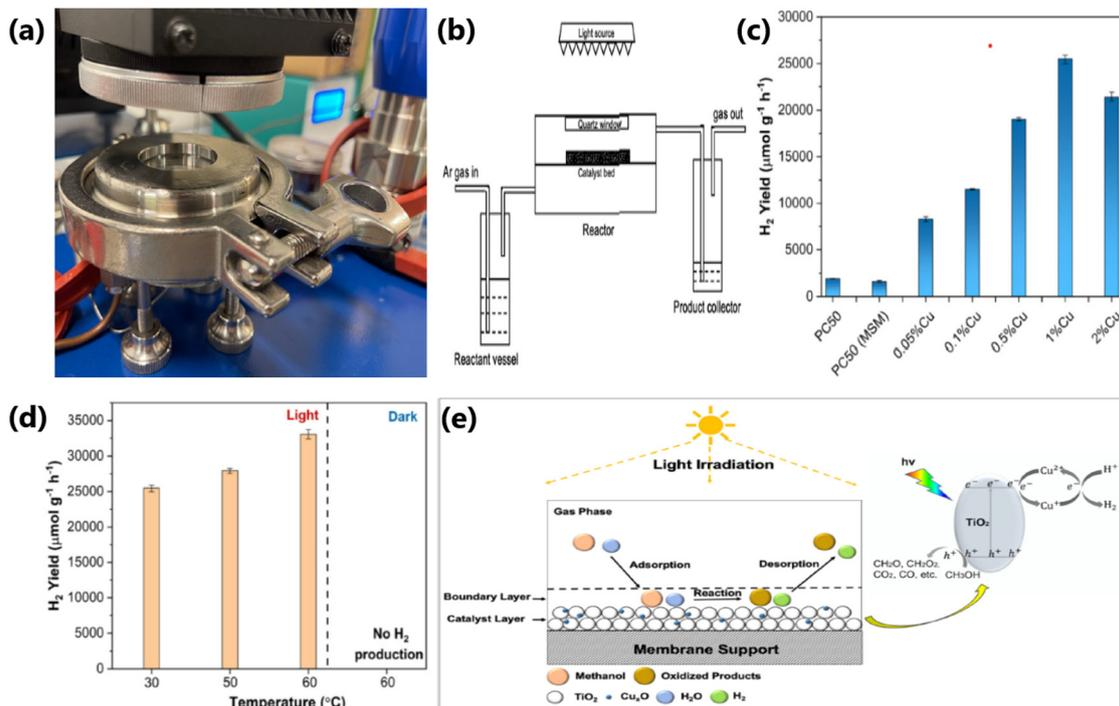
Fig. 29 (a) Digital photograph and (b) schematic diagram of the flow membrane reactor used for photocatalytic methanol dehydrogenation and reforming. (c) H<sub>2</sub> yield obtained with different Cu wt% on PC50. (d) Amount of H<sub>2</sub> produced with 1% Cu/PC50 at different temperatures. (e) Schematic illustration of photocatalytic process on 1% Cu/PC50 in a flow membrane reactor. Reproduced with permission from ref. 226. Copyright ©2022, the Royal Society of Chemistry.
