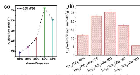
Fig. 20 (a) Variation in the rate of hydrogen production on 50 mg of  $0.5Rh/TSG(TiO_2)$  as a function of calcination temperature (reproduced with permission from ref. 51. Copyright ©2018 Elsevier Ltd). (b) Variation in the rate of hydrogen production as a function of calcination temperature for the Ru (wt% = 8.0)/TiO<sub>2</sub> NB photocatalyst (reproduced with permission from ref. 47. Copyright ©2016, Wiley-VCH).
