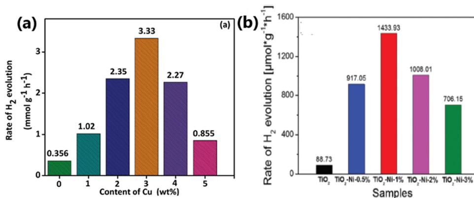
Fig. 26 (a) Variation in the H<sub>2</sub> evolution activity of TiO<sub>2</sub> decorated with different wt% of Cu. Reproduced with permission from ref. 104. Copyright ©2017, the Royal Society of Chemistry. (b) Rate of hydrogen evolution of TiO<sub>2</sub> and TiNi samples with different loadings of Ni. Reproduced with permission from ref. 16. Copyright © 2018, the Royal Society of Chemistry.
