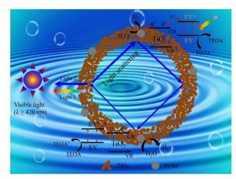
Fig. 13 Mechanism for photocatalytic H<sub>2</sub> evolution over eosin Y-sensitized C-TiO<sub>2</sub> hollow nanoshells with Mie resonance. Reproduced with permission from ref. 74. Copyright ©2021, Elsevier Ltd.
