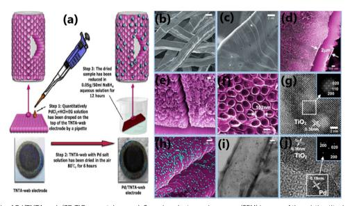
Fig. 24 (a) Synthesis of Pd/TNTA-web (3D TiO<sub>2</sub> nanotube array). Scanning electron microscopy (SEM) images of the pristine titanium-web substrate (b) and (c) and TiO2 nanotubes arrays on the web (d), (e) and (f). HR-TEM image of a nanotube (g), SEM image (h), TEM image (i) and HRTEM image (j) of the TNTA-web with 0.1 mg cm<sup>-2</sup> Pd (0.26 wt%). Reproduced with permission from ref. 205. Copyright ©2018, the Royal Society of Chemistry.
