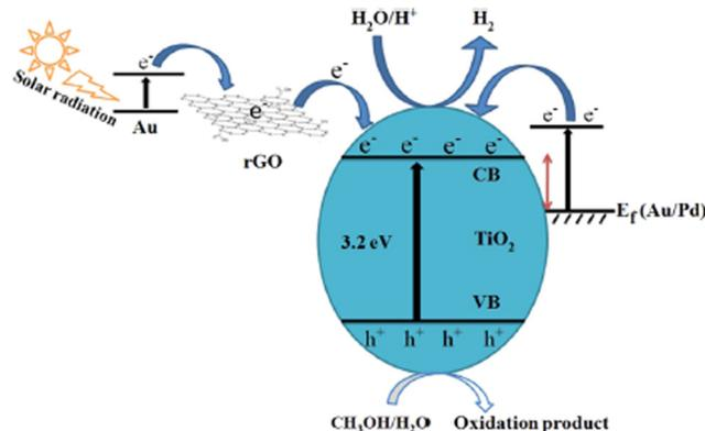
Fig. 14 Schematic illustration of the mechanism of photocatalytic hydrogen evolution from an Au-Pd/rGO/TiO<sub>2</sub> triple composite, in which an SPR electron from Au is transferred to TiO<sub>2</sub> *via* rGO. Reproduced with permission from ref. 66. Copyright ©2019, ACS.
