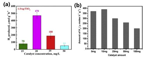
Fig. 25 (a) Photocatalytic hydrogen evolution activity of Ag/TiO<sub>2</sub> by varying the amount of catalyst. Reproduced with permission from ref. 112. Copyright ©2019, Elsevier Ltd. (b) Variation in photocatalytic H<sub>2</sub> evolution rate with respect to the amount of Ni/γ-Al<sub>2</sub>O<sub>3</sub>/CNT-TiO<sub>2</sub> catalyst. Reproduced with permission from ref. 102. Copyright @2017, Elsevier Ltd
