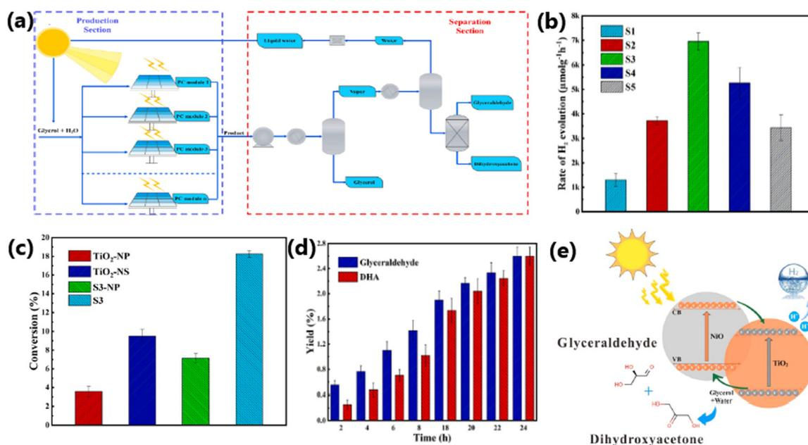
Fig. 28 (a) Schematic illustration of the photocatalytic process. Comparison of H<sub>2</sub> production performance of samples with different nickel loadings (b). (c) Glycerol conversion over different photocatalysts. Yield of liquid products obtained with best-performing catalyst (d) and (e) plausible reaction mechanism. Reproduced with permission from ref. 211. Copyright 2023, Elsevier.
