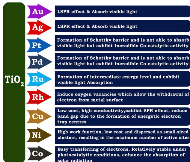
Fig. 5 Schematic representation of various noble metals used for improving the photocatalytic hydrogen evolution activity of TiO<sub>2</sub>.
