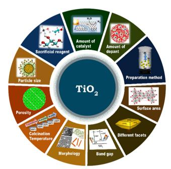
Fig. 15 Schematic representation of the various factors that determine photocatalytic hydrogen evolution activity of TiO2-based photocatalysts
