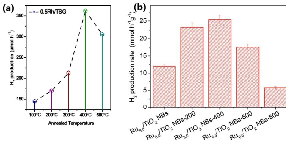
Fig. 20 (a) Variation in the rate of hydrogen production on 50 mg of 0.5Rh/TSG(TiO<sub>2</sub>) as a function of calcination temperature (reproduced with permission from ref. 51. Copyright ©2018 Elsevier Ltd). (b) Variation in the rate of hydrogen production as a function of calcination temperature for the Ru (wt% = 8.0)/TiO<sub>2</sub> NB photocatalyst (reproduced with permission from ref. 47. Copyright ©2016, Wiley-VCH).
