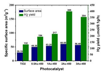
Fig. 19 Amount of hydrogen produced vs. surface area of photocatalyst for Au@TiO2:0.5Au-450, 1Au-450, 2Au-450 and 3A-450 under natural solar light. Adopted from ref. 166. Copyright @2018, the Royal Society of Chemistry
