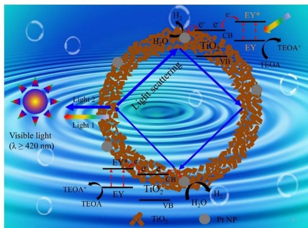
Fig. 13 Mechanism for photocatalytic H<sub>2</sub> evolution over eosin Y-sensitized C-TiO<sub>2</sub> hollow nanoshells with Mie resonance. Reproduced with permission from ref. 74. Copyright ©2021, Elsevier Ltd.
