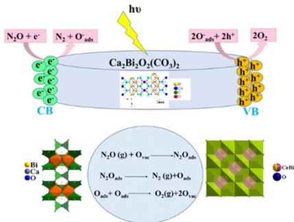
Fig. 7 Plausible mechanism for photocatalytic decomposition of  $N_2O$  using Bi-based photocatalysts.
