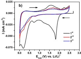
Fig. 8 Cyclic voltammograms of (a) Li-GO-EnBoc and (b) GO electrodes in 1 M LiPF<sub>6</sub> in a 1:1 (v/v) mixture of ethylene carbonate (EC) and dimethyl carbonate (DMC) as the electrolyte with Li as the counter and reference electrode at a scan rate of 0.1 mV s<sup>-1</sup>.
