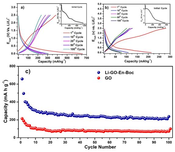
Fig. 7 Charge-discharge profiles for (a) Li-GO-EnBoc and (b) GO electrode cycled at 25 mA g<sup>-1</sup> between 2.5 and 0.005 V vs. Li/Li<sup>+</sup> in 1 M LiPF<sub>6</sub> in a 1:1 (v/v) mixture of ethylene carbonate (EC) and dimethyl carbonate (DMC) as the electrolyte. (c) Variation in discharge capacity vs. cycle number for GO and Li-GO-EnBoc.
