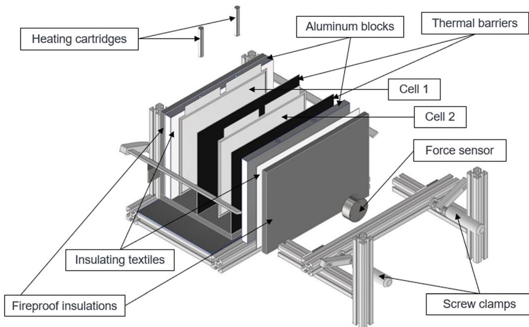
Fig. 2 Explosion view of the experimental setup. The setup is insulated from the outside by fire protection panels and a force sensor is installed on the aluminum profile to determine the contact pressure.
