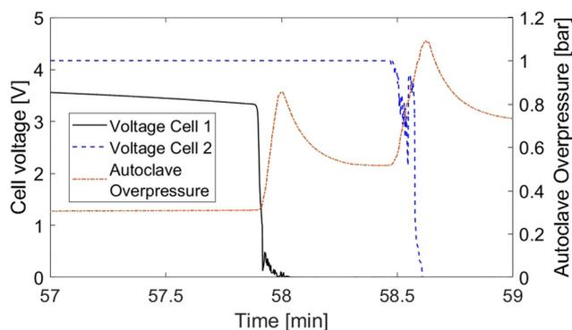
**Fig. 5** Cell voltages and autoclave overpressure during experiment 4.
