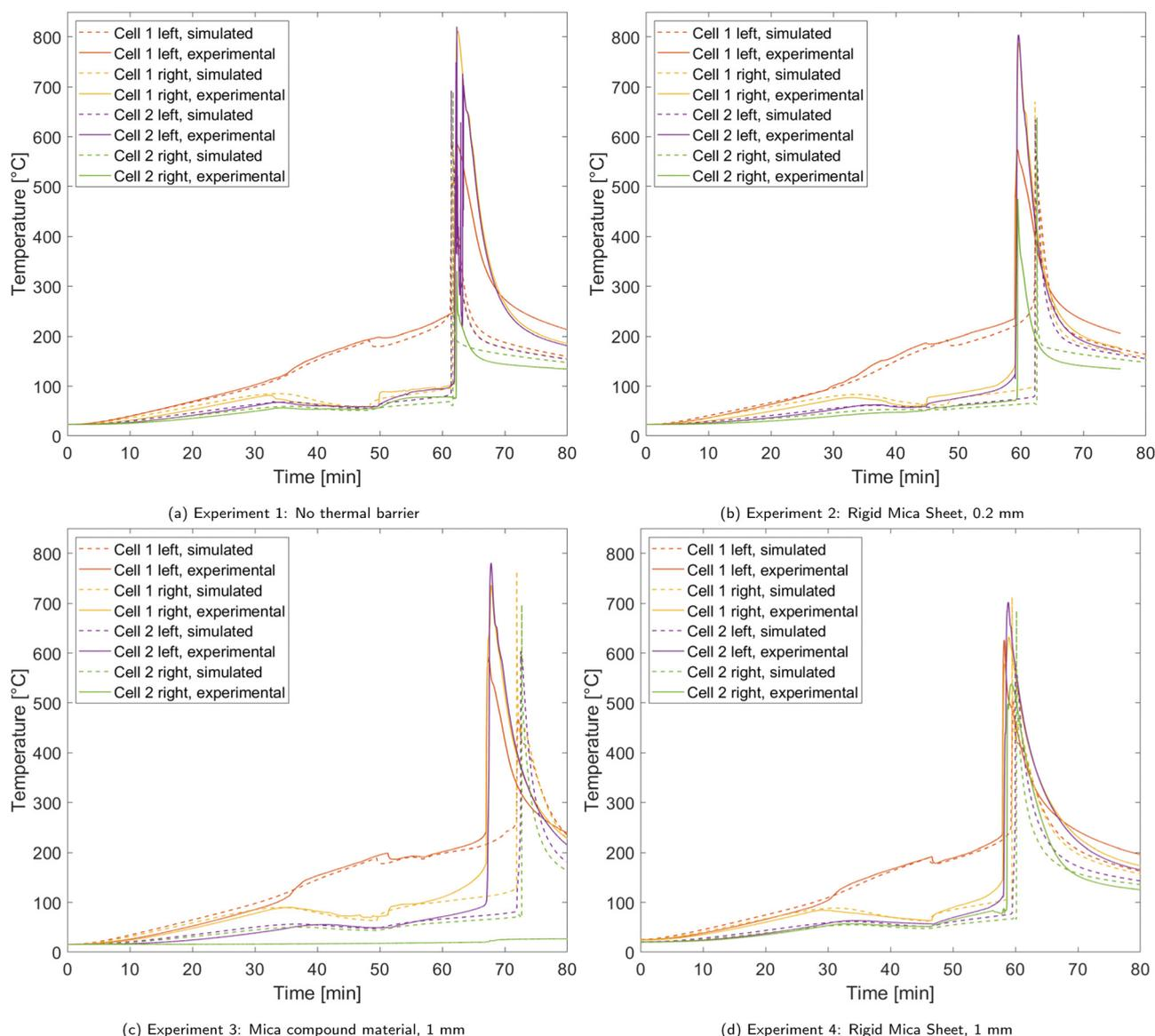
**Fig. 3** Comparison of temperature curves between experiments 1 to 4 and the according simulations. Temperature is measured on both sides of each cell. In (c): please note that the thermocouple at 'cell 2, right experimental' failed during the experiment and therefore the temperature curve is not considered further in the analysis of the results. In (a): the signal for thermocouple 'cell 2, left experimental' scatters due to a brief signal disruption.
