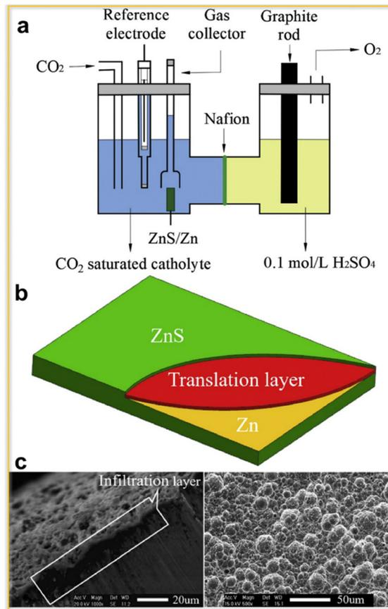
Fig. 3 (a) An organic electrolyte-based two-compartment electrolysis cell, (b) an infiltration layer schematic and (c) a scanning electron micrograph of a ZnS electrode.<sup>75</sup>
