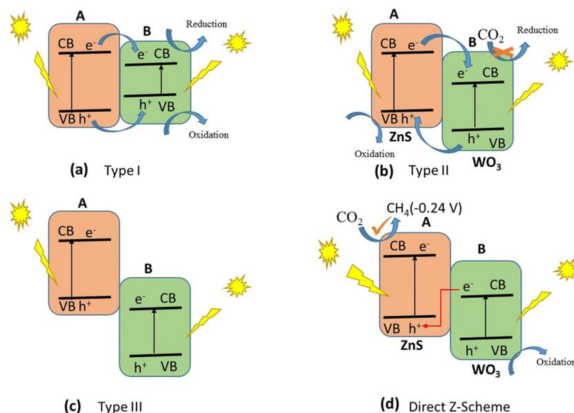
Fig. 8 The mechanism of photocatalytic CO<sub>2</sub> reduction on ZnS/WO<sub>3</sub> heterojunctions as they respond to light radiation is depicted schematically.
