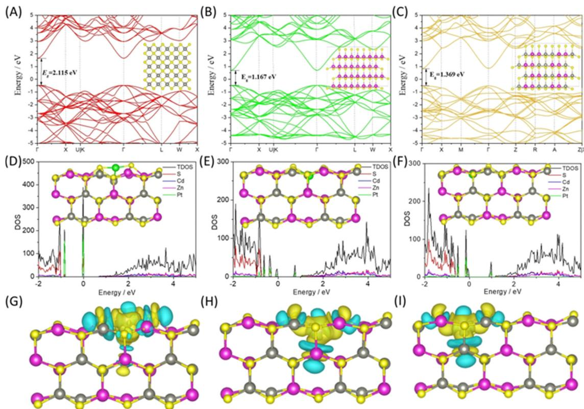
Fig. 12 The electronic structures of (A) ZnS, (B) CdS, and (C)  $\text{Zn}_x\text{Cd}_{1-x}\text{S}$  are shown (the gray, pink, and yellow spheres represent Zn, Cd, and S atoms, respectively). The work functions of (D)  $\text{Zn}_x\text{Cd}_{1-x}\text{S-Pt1}$ , (E)  $\text{Zn}_x\text{Cd}_{1-x}\text{S-Pt1}$  (Zn), (F)  $\text{Zn}_x\text{Cd}_{1-x}\text{S-Pt1}$  (Cd). (G), (H), and (I) indicate the DOSs and charge density differences.<sup>139</sup>
