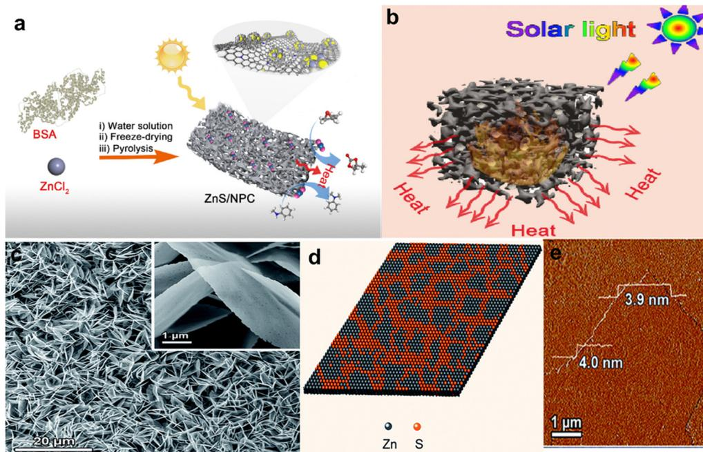
Fig. 5 (a) Schematic illustration of the preparation of ZnS/NPC-X for catalytic conversion of CO<sub>2</sub>, by pyrolyzing protein-Zn(II) networks. (b) Schematic illustration of the photothermal effect of ZnS/NPC-X (c)–(e) Characterization of S-Zn-S NSs. (c) SEM image; inset shows a typical single nanosheet. (d) Schematic map of the structure of S-Zn-S NSs. (e) AFM image.<sup>73</sup>
