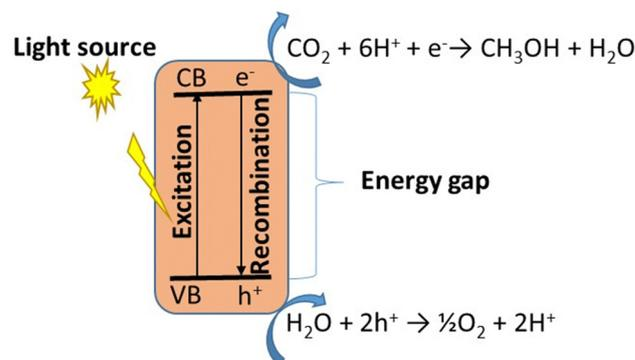
Fig. 7 Schematic representation of a single photocatalyst.
