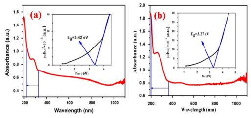
Fig. 4 The UV analysis results for the MWCNT synthesized at (a) 650  $^{\circ}$ C and (b) 750  $^{\circ}$ C.
