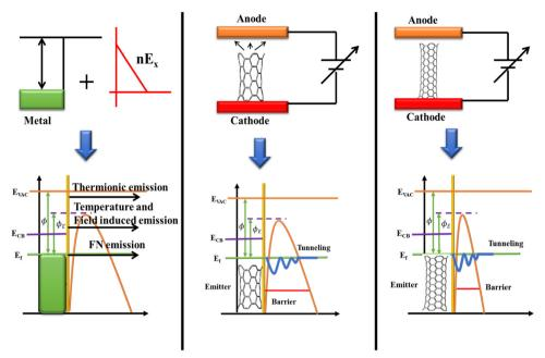
Fig. 10 The field emission mechanism in the presence of the electric field and FE enhancement with the increasing tube length.
