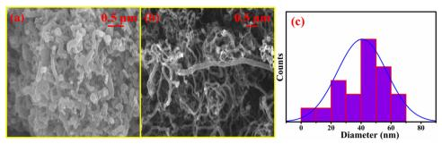
Fig. 2 (a) and (b) The SEM images of the MWCNTs grown at 650 °C and 750 °C, (c) the average diameters.
