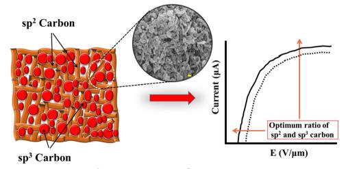
Fig. 9 The transport of electrons between the sp<sup>2</sup> cluster embedded in the sp<sup>3</sup> rich matrix.
