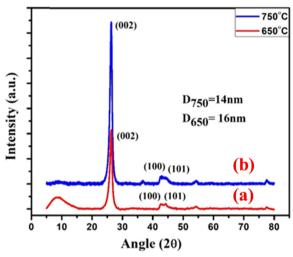
Fig. 5  $\,$  The XRD analysis of the MWCNTs synthesized at (a) 650  $^{\circ}\text{C}$  and (b) 750  $^{\circ}\text{C}.$
