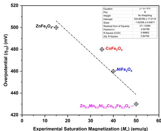
Fig. 10 Alkaline OER overpotential  $\eta_{10}$  needed to drive current density  $j = 10$  mA cm<sup>-2</sup> as a function of saturation magnetization of the synthesized ferrite catalysts.
