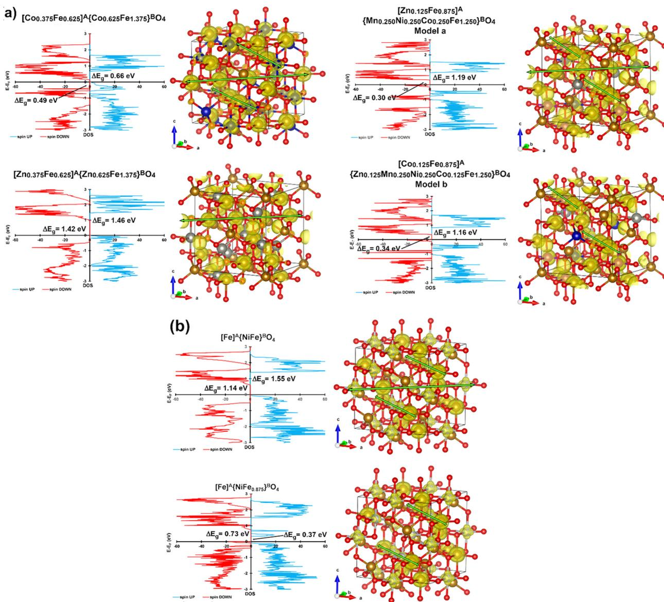
Fig. 5 (a) Density of states (DOS, left) and  $\alpha - \beta > 0$  spin density (spin up,  $0.04 a_0^{-3}$ , right) for the most stable ground states of partially inverse spinel model a and model b of  $Zn_{0.2}Mn_{0.2}Ni_{0.2}Co_{0.2}Fe_{2.2}O_4$ , and (b) DOS (left) and  $\alpha - \beta > 0$  spin density (spin up,  $0.04 a_0^{-3}$ , right) for the most stable ground states of perfect  $NiFe_2O_4$  and defective  $NiFe_{2-x}O_4$ . Possible spin channels are marked with green arrows.
