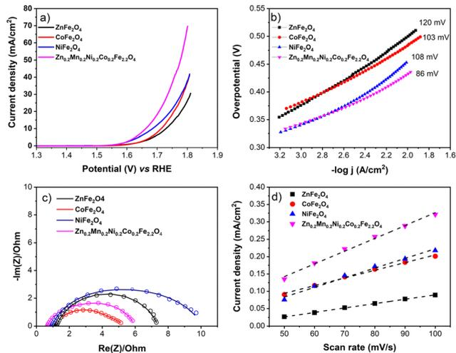
**Fig. 7** (a) Representative LSV voltammograms recorded at the 5 mV s<sup>-1</sup> scan rate and (b) Tafel plots extracted from the respective LSV curves; (c) Nyquist plot; (d) capacitive current density as a function of scan rate for the synthesized ZnFe<sub>2</sub>O<sub>4</sub>, CoFe<sub>2</sub>O<sub>4</sub>, NiFe<sub>2</sub>O<sub>4</sub>, and Zn<sub>0.2</sub>Mn<sub>0.2</sub>Ni<sub>0.2</sub>Co<sub>0.2</sub>Fe<sub>2.2</sub>O<sub>4</sub> catalysts.
