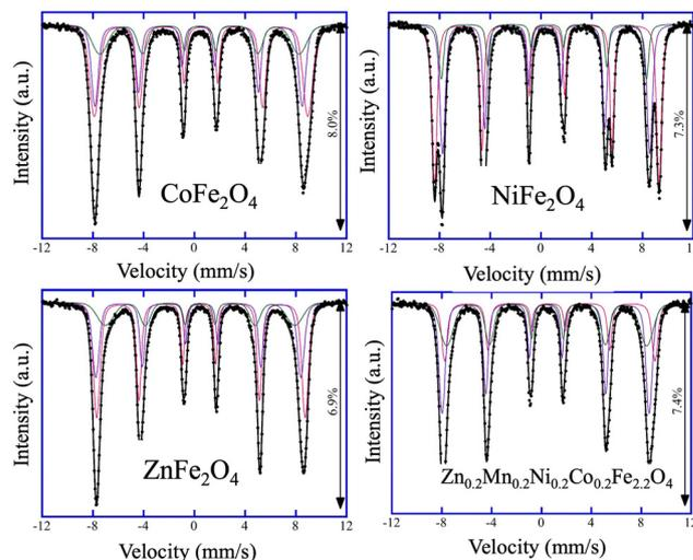
Fig. 1 Mössbauer spectra of  $CoFe_2O_4$ ,  $NiFe_2O_4$ ,  $ZnFe_2O_4$ , and high-entropy  $Zn_{0.2}Mn_{0.2}Ni_{0.2}Co_{0.2}Fe_{2.2}O_4$  catalysts collected at 6 K. Experimental data: black circles. Calculated spectrum: black line.  $Q_1$ ,  $Q_2$ , and  $Q_3$  components: red, violet, and green, respectively.
