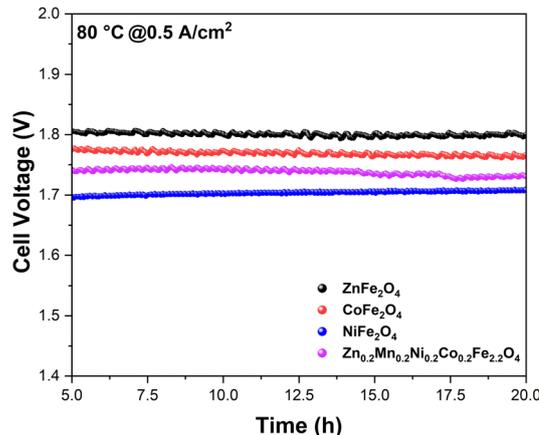
**Fig. 9** Cell-voltage changes at a constant current density of 0.5 A cm<sup>-2</sup> as a function of testing time for the AEMEL cells with the synthesized ZnFe<sub>2</sub>O<sub>4</sub>, CoFe<sub>2</sub>O<sub>4</sub>, NiFe<sub>2</sub>O<sub>4</sub>, and Zn<sub>0.2</sub>Mn<sub>0.2</sub>Ni<sub>0.2</sub>Co<sub>0.2</sub>Fe<sub>2.2</sub>O<sub>4</sub> anode catalysts, recorded at 80 °C under atmospheric pressure in 1 M KOH electrolyte.
