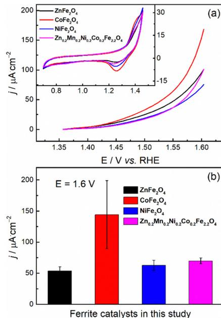
Fig. 6 (a) Representative positive going linear sweep voltammograms at OER potentials and (b) the current densities (normalized by ECSA) at  $1.6 \text{ V}_{\text{RHE}}$  towards the OER for the synthesized catalysts. The corresponding basic cyclic voltammograms are given as the inset in (a).
