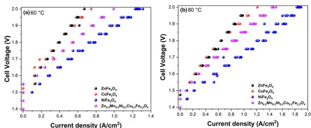
**Fig. 8** Polarization curves of AEMEL cells with the synthesized ZnFe<sub>2</sub>O<sub>4</sub>, CoFe<sub>2</sub>O<sub>4</sub>, NiFe<sub>2</sub>O<sub>4</sub>, and Zn<sub>0.2</sub>Mn<sub>0.2</sub>Ni<sub>0.2</sub>Co<sub>0.2</sub>Fe<sub>2.2</sub>O<sub>4</sub> anode catalysts recorded at 60 °C (a) and 80 °C (b) under atmospheric pressure in 1 M KOH electrolyte.
