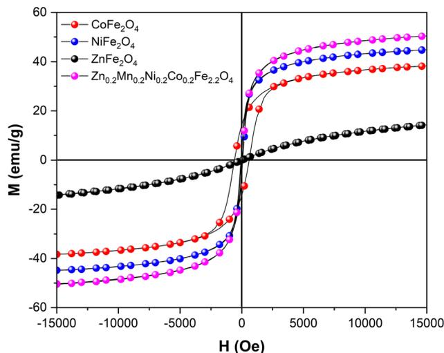
**Fig. 4** Room temperature  $M(H)$  dependence data for the synthesized catalysts.
