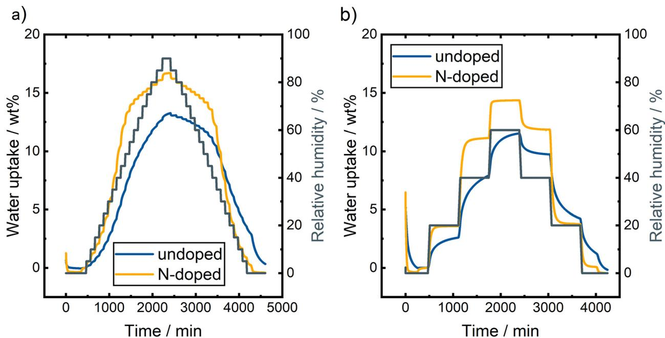
Fig. 6 DVS measurements of undoped and N-doped BC applying different measurement procedures with (a) 5% RH steps up to 90% RH and (b) 20% RH steps with longer duration up to 60% RH.
