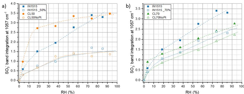
Fig. 9 Hydration-dependent characteristic functions of the ionomer. Band integration at  $1057\text{ cm}^{-1}$  (band normalized to ionomer backbone band at  $1570\text{ cm}^{-1}$ , integration subtracted from its value at 0% RH) versus humidity for CL50 and CL50NoPt (a), and CL70 and CL70NoPt (b), compared to the IN1515 membrane (IN1515\_50% and IN1515\_70% correspond to 50% and 70% of the integration values within these bands, respectively).
