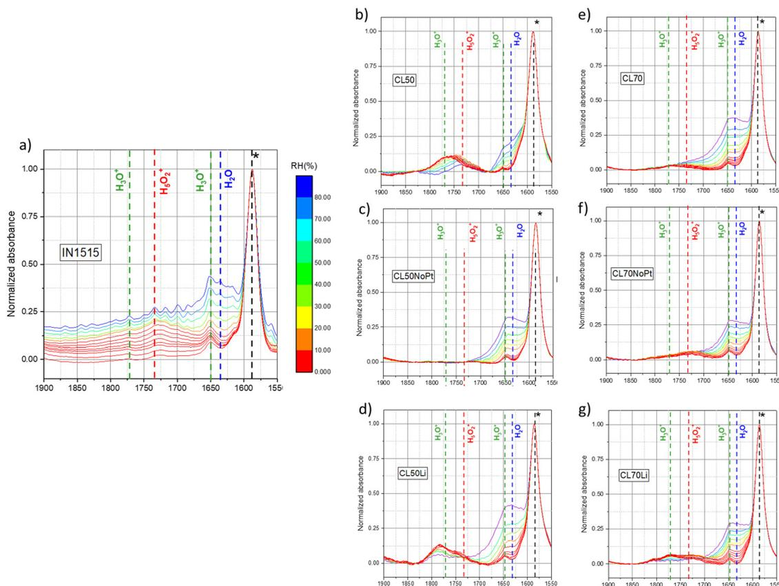
Fig. 6 *In situ* MIR spectra of (a) IN1515, (b) CL50, (c) CL50NoPt, (d) CL50Li, (e) CL70, (f) CL70NoPt, (g) CL70Li in the range 1500–1900  $\text{cm}^{-1}$  (spectra normalized to ionomer backbone band at 1588  $\text{cm}^{-1}$ ): the characteristic bands of specific species ( $\text{H}_2\text{O}$ ,  $\text{H}_3\text{O}^+$ ,  $\text{H}_5\text{O}_2^+$ ) relative to the exposition of materials to humidity are indicated by dotted lines. (see Fig. S2 and S3, ESI†).
