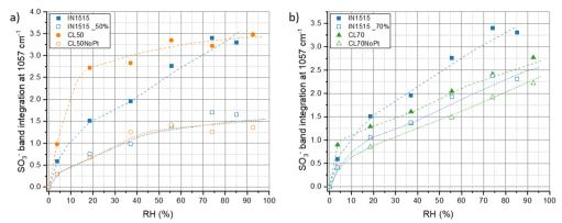
Fig. 9 Hydration-dependent characteristic functions of the ionomer. Band integration at 1057 cm<sup>-1</sup> (band normalized to ionomer backbone band at 1570 cm<sup>-1</sup>, integration subtracted from its value at 0% RH) *versus* humidity for CL50 and CL50NoPt (a), and CL70 and CL70NoPt (b), compared to the IN1515 membrane (IN1515\_50% and IN1515\_70% correspond to 50% and 70% of the integration values within these bands, respectively).
