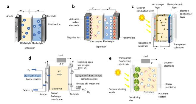
Fig. 20 Typical structures of the four most common applications of polymer electrolytes. Schematic of (a) a battery; (b) a double-layer capacitor; (c) an eletrochromic devices, (d) a hydrogen fuel cell; and (e) a dye-sensitized solar cell
