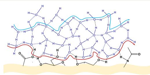
Fig. 8 Suggested pathways of proton diffusion *via* a Grotthuss-like mechanism. Red pathway: proton diffusion involving water molecules and functional groups attached to the polysaccharide chain. Blue pathway: proton diffusion solely *via* water molecules situated within the HA biomolecule. Adapted from ref. 125; copyright © 2021 The Authors; published by The Royal Society of Chemistry. This work is licensed under a Creative Commons Attribution 3.0 CC-BY Unported License.
