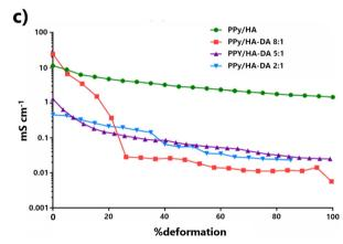
Fig. 13 (a) Conductivities of PPy/HA and PPy/(HA–DA) films on a poly(dimethylsiloxane) substrate. (b) Conductivities of PPy/HA and PPy/(HA–DA) 8:1 films under different humidity conditions. (c) Conductivity as a function of applied stress; conductivity measurements are shown as the mean and standard deviation of n=3. Reproduced, with adaptations, from ref. 233 with permission from Elsevier; copyright © 2017 Elsevier B.V.
