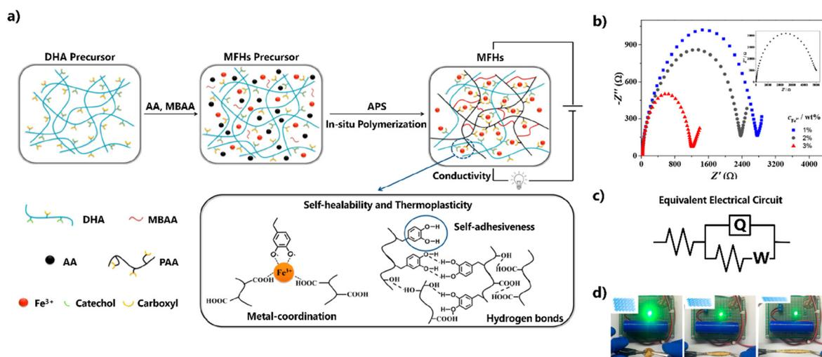
**Fig. 19** (a) Schematic of the synthetic process for the multifunctional conductive hydrogels and the corresponding interactions inside multifunctional networks; (b) electrochemical impedance plot of the hydrogels with different  $c(\text{Fe}^{3+})$ , and (c) the corresponding equivalent electrical circuit; and (d) images of strain-dependent conductivity performance of the hydrogels. Reproduced from ref. 436 with permission from The American Chemical Society. Copyright © 2019.
