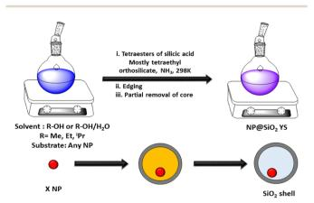
Fig. 7 Schematic design of core-shell/yolk-shell formation via the Stö-
