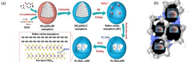
Fig. 5 (a) Illustration of the preparation process of the FL-MoS $_{2-x}$ @HC matrix. (b) Molecular assembly into the molecular porous template. Reprinted with permission from ref. 176.  $\bigcirc$ 2021, Wiley-VCH GmbH.
