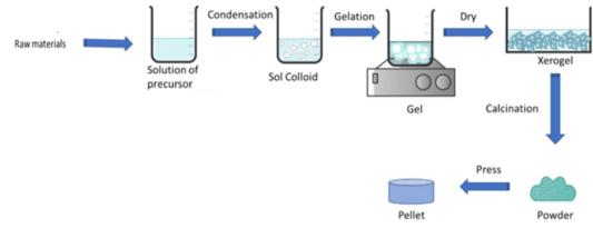
Schematic view of the sol-gel method. 189 Reprinted with permission from ref. 189. Copyright ©2020, Elsevier Inc.
