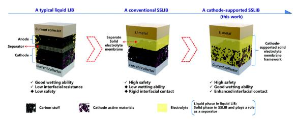
Fig. 8 Schematic of the novel cathode-supported SSLIB in comparison with a conventional rigid SSLIB and a typical liquid LIB. (Reproduced with permission from ref. 43).
