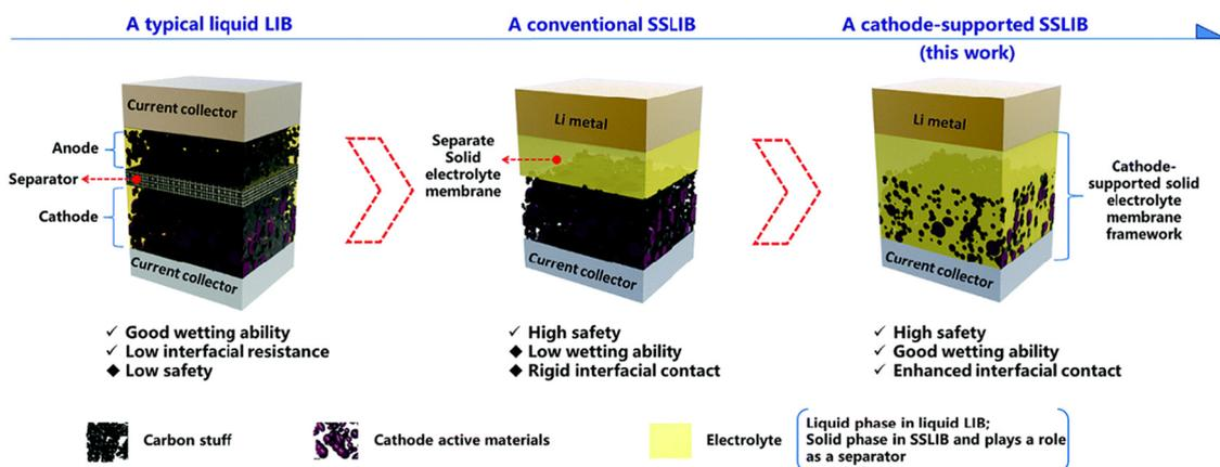
**Fig. 8** Schematic of the novel cathode-supported SSLIB in comparison with a conventional rigid SSLIB and a typical liquid LIB. (Reproduced with permission from ref. 43).
