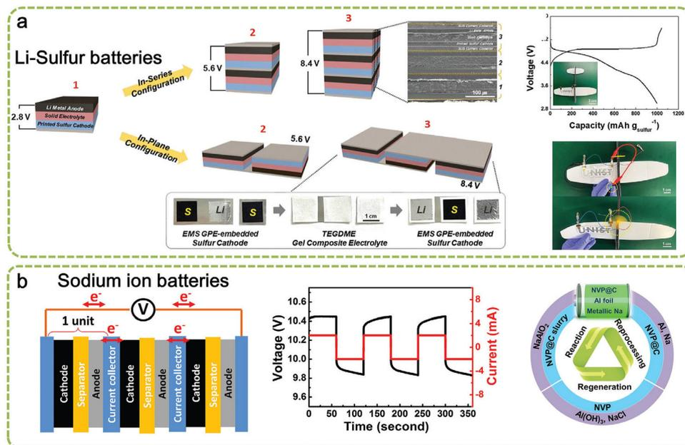
**Fig. 15** Fabrication and characterization of the printed bipolar ASSLSBs. (a) Schematic representation depicting the fabrication procedure of the printed bipolar ASSLSBs, along with the SEM image (in-series configuration) and photographs (in-plane configurations). (b) Charge/discharge profiles of the printed bipolar ASSLSBs during the 1st cycle (at a charge/discharge current density of 0.1C/0.1C) as a function of cell number. (Reproduced with permission from ref. 73).
