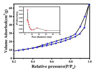
Fig. 6 BET surface area analysis of a  $Cu_2ZnSnS_4$  nanoparticle. The inset depicts the Barrett–Joyner–Halenda pore size distribution curves.
