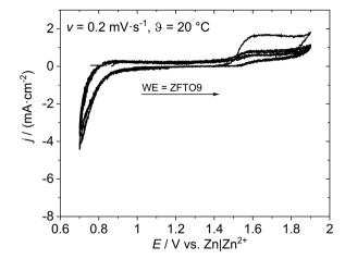
Fig. 6 Cyclovoltammetry measurement of ZFTO9 || Sn.
