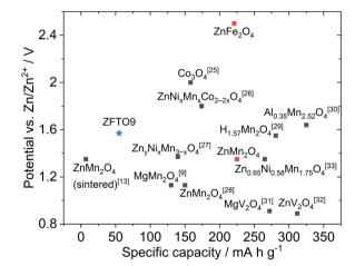
Specific capacity and potential of ZFTO9 (blue star) in comparison with the highest theoretically possible values for ZnMn<sub>2</sub>O<sub>4</sub> and ZnFe<sub>2</sub>O<sub>4</sub> (red squares) and experimentally determined values for different oxide spinel materials from ref. 9, 13 and 25-33.
