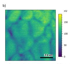
Fig. 5 (a) Work function ( $\phi$ ) measurements of ZFO, ZFTO7 and ZFTO13 (black squares) and data for the band gap energies ( $E_0$ ) calculated from the Tauc plot for all samples except ZFTO25 (red circles). Error bars of work function are standard deviation from the average value. (b) Exemplary KPFM image of ZFO with grain boundaries showing lower surface potential (blue) than grain interior (green).
