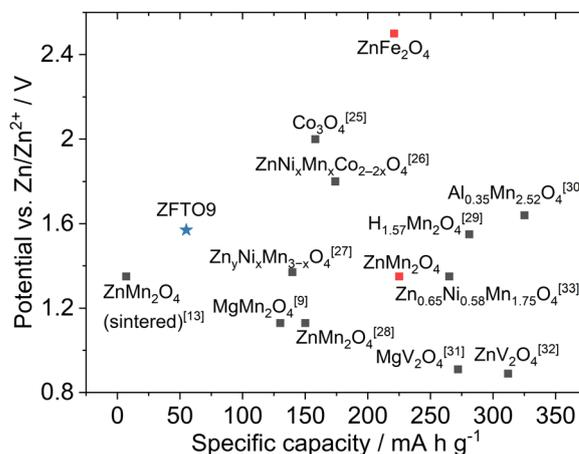
Fig. 9 Specific capacity and potential of ZFTO9 (blue star) in comparison with the highest theoretically possible values for  $\text{ZnMn}_2\text{O}_4$  and  $\text{ZnFe}_2\text{O}_4$  (red squares) and experimentally determined values for different oxide spinel materials from ref. 9, 13 and 25–33.
