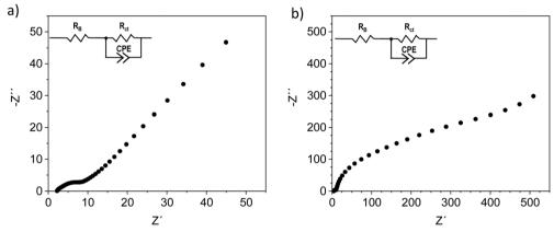
Impedance measurement with (a) ZFTO9||Sn and (b) ZFTO13||Sn. The error of fitting was below 3% using the given equivalent circuit.
