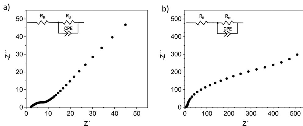
Fig. 8 Impedance measurement with (a) ZFTO9||Sn and (b) ZFTO13||Sn. The error of fitting was below 3% using the given equivalent circuit.
