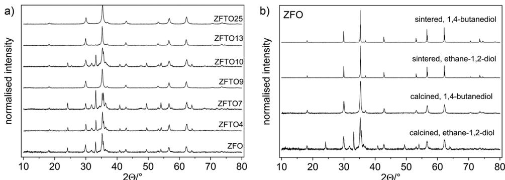
Fig. 1 (a) PPXRD measurements of the calcined samples. ZFTO9, ZFTO13 and ZFTO25 show only very small amounts of secondary phases. (b) Comparison between the calcined and sintered pure  $\text{ZnFe}_2\text{O}_4$  produced either with ethane-1,2-diol or 1,4-butanediol.
