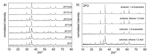
Fig. 1 (a) PPXRD measurements of the calcined samples. ZFTO9, ZFTO13 and ZFTO25 show only very small amounts of secondary phases. (b) Comparison between the calcined and sintered pure ZnFe<sub>2</sub>O<sub>4</sub> produced either with ethane-1,2-diol or 1,4-butanediol.
