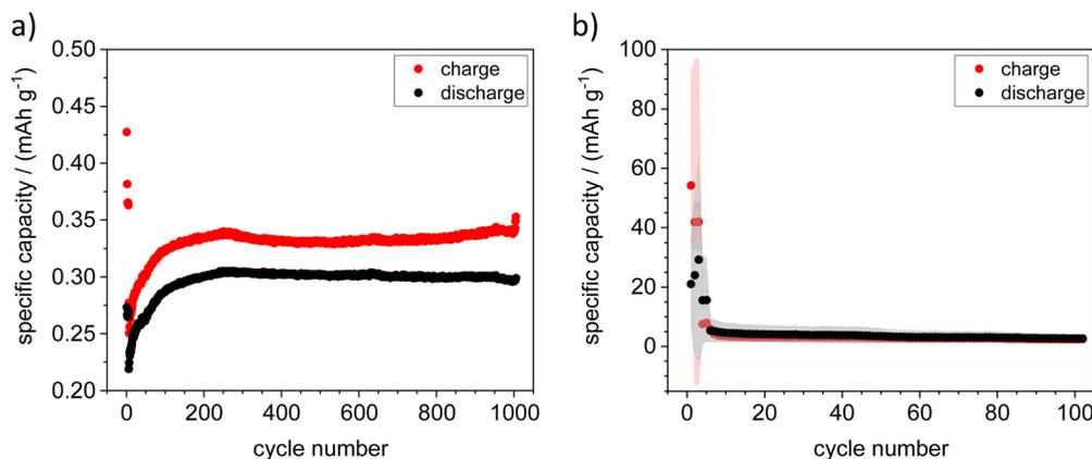
Fig. 7 Galvanostatic cycling experiments with ZFTO9||Zn with (a) Zn metal sheet at 0.1C and (b) Zn on Ti foil (sputtered), which showed an average initial specific capacity of  $55 \text{ mA h g}^{-1}$  at 0.1C. Points are averaged values, red or gray areas around the points show the scatter of the individual measurements.
