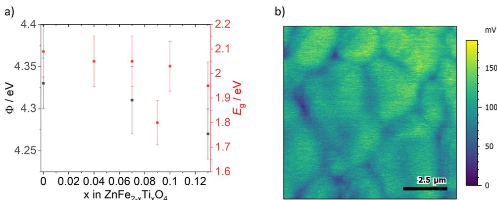
**Fig. 5** (a) Work function ( $\phi$ ) measurements of ZFO, ZFTO7 and ZFTO13 (black squares) and data for the band gap energies ( $E_g$ ) calculated from the Tauc plot for all samples except ZFTO25 (red circles). Error bars of work function are standard deviation from the average value. (b) Exemplary KPFM image of ZFO with grain boundaries showing lower surface potential (blue) than grain interior (green).
