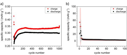
Fig. 7 Galvanostatic cycling experiments with ZFTO9 | Zn with (a) Zn metal sheet at 0.1C and (b) Zn on Ti foil (sputtered), which showed an average initial specific capacity of 55 mA h  $\text{g}^{-1}$  at 0.1 C. Points are averaged values, red or gray areas around the points show the scatter of the individual measurements.
