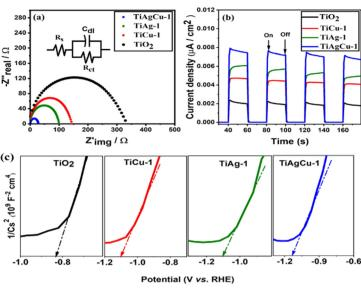
Fig. 4 (a) Nyquist plots, (b) transient photocurrent responses under light illumination conditions, and (c) Mott-Schottky plot of TiO2, TiAg-1, TiCu-1, and TiAgCu-1. The electrochemical experiments were carried out in 0.5 M Na<sub>2</sub>SO<sub>4</sub> (pH = 7.5) at a potential of 1.23 V (vs. NHE)
