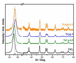
Fig. 1 Wide angle XRD patterns of mesoporous TiO<sub>2</sub>, Ag/TiO<sub>2</sub> (TiAg-1), Cu/TiO<sub>2</sub> (TiCu-0.5) and TiAgCu-1 nanocomposites. A significant shift and broadening of the (101) diffraction feature is observed with TiAq-1 and TiAgCu-1. All the diffraction features are attributed to the anatase phase of TiO<sub>2</sub>.
