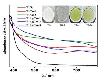
Fig. 3 UV Visible absorption spectra of mesoporous TiO<sub>2</sub> and representative samples of metal integrated TiO2 nanocomposites
