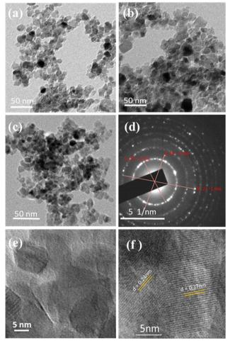
Fig. 2 TEM images of (a)  $TiO_2$ , (b) TiCu-1, and (c) TiAg-1; (d) SAED pattern of TiAgCu-1, and HRTEM images of (e) TiAgCu-1 and (f) the lattice fringe spacing in TiAgCu-1. Ag and Cu integration on TiO2 and the formation of a metal-semiconductor Schottky junction between Ag/Cu and TiO2 is evident from the d-values (0.24 nm for Ag/Cu alloy formation and 0.37 for TiO<sub>2</sub>) observed in the HRTEM image in (f).
