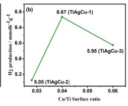
Fig. 8 (a) Variation of rate of hydrogen production with Ag/Ti surface ratio. (b) Variation of rate of hydrogen evolution with Cu/Ti surface ratio.
