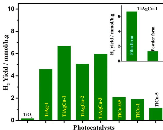
Fig. 6 Photocatalytic H<sub>2</sub> production activity of mesoporous TiO<sub>2</sub>, Ag/TiO<sub>2</sub>, Cu/TiO<sub>2</sub> and Ag-Cu/TiO<sub>2</sub> nanocomposites, measured in thin film form under direct sunlight. Inset shows a comparison of the solar hydrogen generation activity for the thin film and powder catalysts of TiAgCu-1.
