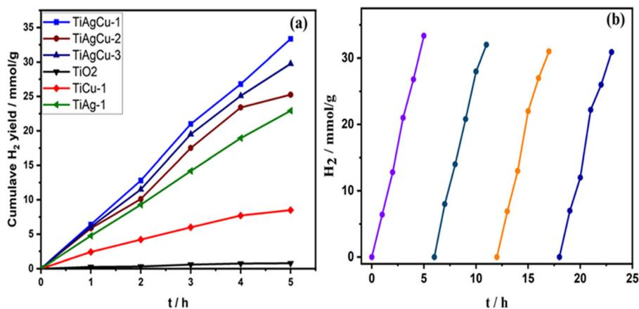
Fig. 7 (a) Time on stream dependence of solar hydrogen production of the mesoporous TiO<sub>2</sub>, TiAg-1, TiCu-1 and TiAgCu nanocomposites (in thin film form) from solar hydrogen evolution. (b) Solar hydrogen production as a function of time with repeated cycles of operation for TiAgCu-1 in direct sunlight.
