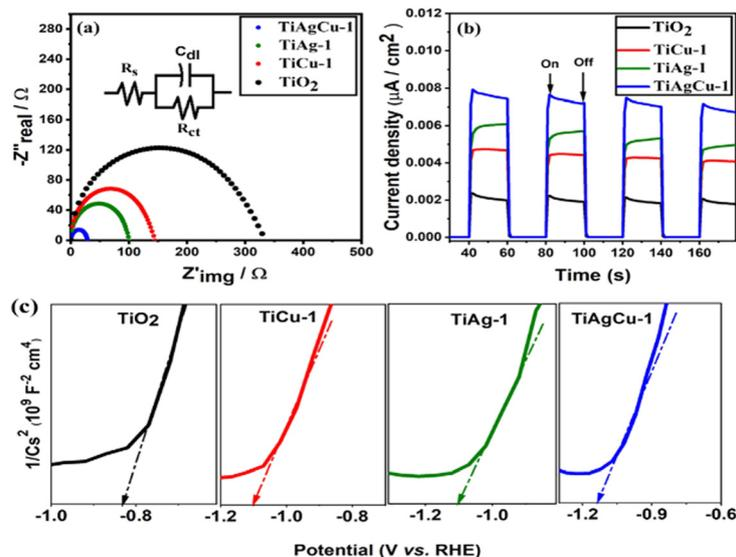
Fig. 4 (a) Nyquist plots, (b) transient photocurrent responses under light illumination conditions, and (c) Mott–Schottky plot of TiO<sub>2</sub>, TiAg-1, TiCu-1, and TiAgCu-1. The electrochemical experiments were carried out in 0.5 M Na<sub>2</sub>SO<sub>4</sub> (pH = 7.5) at a potential of 1.23 V (vs. NHE).
