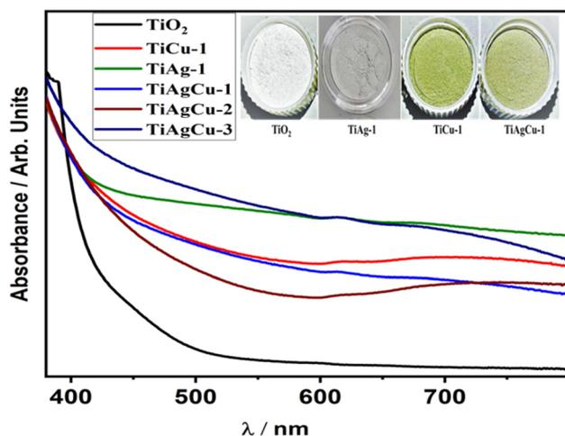
Fig. 3 UV Visible absorption spectra of mesoporous TiO<sub>2</sub> and representative samples of metal integrated TiO<sub>2</sub> nanocomposites.
