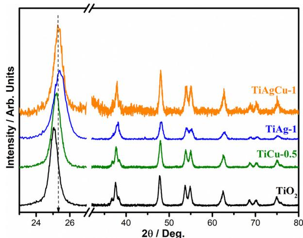
**Fig. 1** Wide angle XRD patterns of mesoporous  $\text{TiO}_2$ ,  $\text{Ag}/\text{TiO}_2$  (TiAg-1),  $\text{Cu}/\text{TiO}_2$  (TiCu-0.5) and TiAgCu-1 nanocomposites. A significant shift and broadening of the (101) diffraction feature is observed with TiAg-1 and TiAgCu-1. All the diffraction features are attributed to the anatase phase of  $\text{TiO}_2$ .
