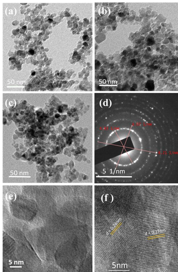
**Fig. 2** TEM images of (a)  $\text{TiO}_2$ , (b) TiCu-1, and (c) TiAg-1; (d) SAED pattern of TiAgCu-1, and HRTEM images of (e) TiAgCu-1 and (f) the lattice fringe spacing in TiAgCu-1. Ag and Cu integration on  $\text{TiO}_2$  and the formation of a metal-semiconductor Schottky junction between Ag/Cu and  $\text{TiO}_2$  is evident from the  $d$ -values (0.24 nm for Ag/Cu alloy formation and 0.37 nm for  $\text{TiO}_2$ ) observed in the HRTEM image in (f).
