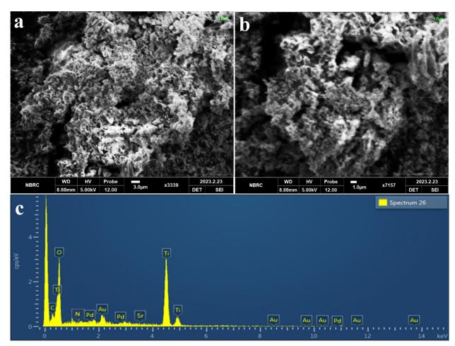
Fig. 3 SEM images of Pd-SrO@TiO $_2$ /gCN at (a) 3.0  $\mu$ m and (b) 1.0  $\mu$ m; (c) EDX of Pd-SrO@TiO $_2$ /gCN.
