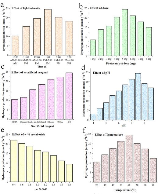
Fig. 7 Representing the factors effecting the rate of hydrogen production (mmol  $g^{-1} h^{-1}$ ), (a) effect of light intensity, (b) effect of dose, (c) effect of sacrificial reagent, (d) effect of pH, (e) effect of w% metal oxide loading, and (f) effect of temperature.
