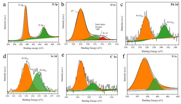
Fig. 4 Pd-SrO@TiO<sub>2</sub>/gCN XPS spectra at the core level (a) Ti 2p, (b) O 1s, (c) Pd 3d, (d) Sr 3d, (e) C 1s (f) N 1s.
