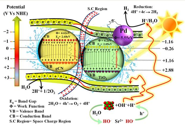
Fig. 6 The mechanism of  $H_2$  evolution through solar water splitting using Pd-SrO@TiO<sub>2</sub>/gCN
