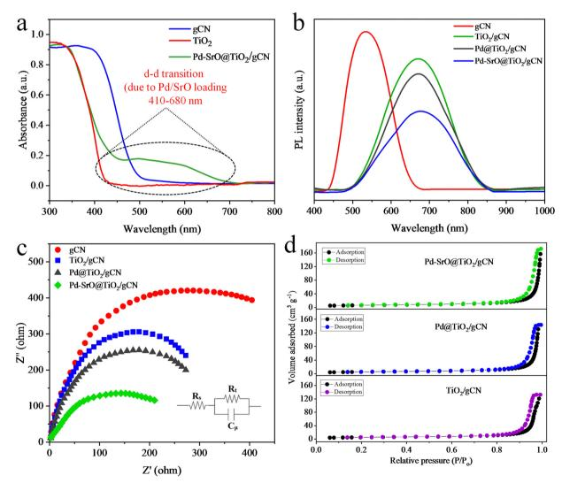
Fig. 2 (a) UV-DRS spectra of TiO2, gCN and Pd-SrO@TiO2/gCN; (b) PL spectra at the excitation wavelength of 325 nm; (c) EIS results of gCN, TiO2/gCN, Pd@TiO2/gCN, and Pd-SrO@TiO2/gCN; (d) BET analyses of TiO2/gCN, Pd@TiO2/gCN and Pd-SrO@TiO2/gCN.
