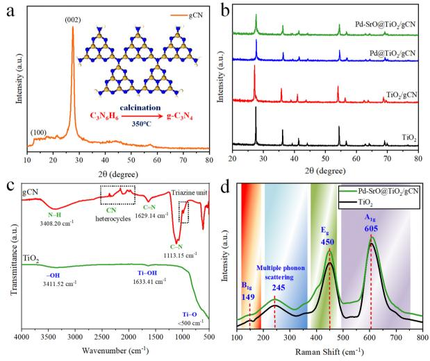
Fig. 1 (a) XRD pattern of gCN; (b) XRD patterns of TiO<sub>2</sub>, TiO<sub>2</sub>/gCN, Pd@TiO<sub>2</sub>/gCN, and Pd-SrO@TiO<sub>2</sub>/gCN; (c) FTIR patterns of TiO<sub>2</sub> and gCN; (d) Raman bands of TiO<sub>2</sub> and Pd-SrO@TiO<sub>2</sub>/gCN.
