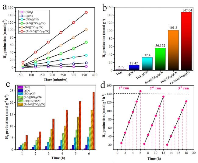
Fig. 5 Hydrogen generation activity results: (a)  $H_2$  generation at the rate of (mmol  $g^{-1}$ ), with (b) representing the total hydrogen production percentage by each photocatalyst; (c)  $H_2$  generation at the rate of (mmol  $g^{-1}$   $h^{-1}$ ) by the as-synthesized photocatalysts; (d) a 3-run recyclability test of Pd-SrO@TiO<sub>2</sub>/gCN.
