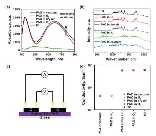
Fig. 2 (a) UV-Vis absorption spectra, and (b) FTIR of Spiro-OMeTAD films PAO in different ambient conditions, (c) testing device structure for conductivity measurements, and (d) effective conductivity of Spiro-OMeTAD PAO in different media measured by a four-point probe
