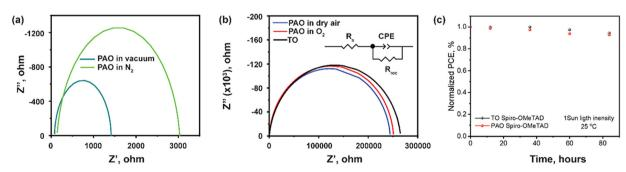
Fig. 6 (a) Nyquist plot for the devices with PAO Spiro-OMeTAD in vacuum and  $N_2$ , and (b) Nyquist plot for the devices with TO and PAO Spiro-OMeTAD in  $O_2$  and dry air. (c) Light soaking stability test for the TO and PAO Spiro-OMeTAD based perovskite solar cells with a carbon electrode.
